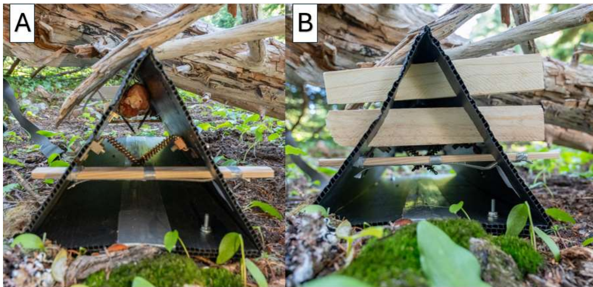
Figure 4. We used a ground cubby at each hair snare transect station. Each side of the cubby measured 20 cm with a length of 80cm. The cubby was held together with a bolt and nut at each end. A) We tied a chicken leg to the center of the cubby, and secured gun brushes and a slat with a glue strip in place to trap hair. The glue strip was held in place with strips of duct tape here, but we later found stapling to be the best method. B) We inserted wooden slats at the end of the cubby to force a marten to go under the glue strip to enter and exit the cubby. Photos by B. Wymer.
