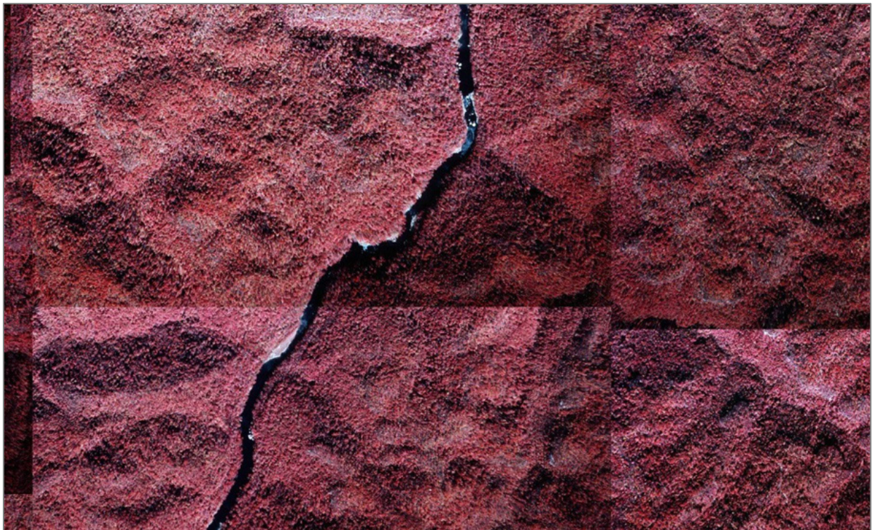
Figure 8. A mosaic of orthorectified 1:16,000-scale photographs of BISO was created for quality assurance and checking and to provide an image backdrop for the GIS database. The ground pixel dimension is 0.75 m.
