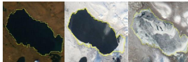
Figure 3. Examples of metric thresholds from Lake Becharof. MODIS true color images with no ice cover on October 11, 14% on December 23, and 92% (freeze-over) on February 15.
