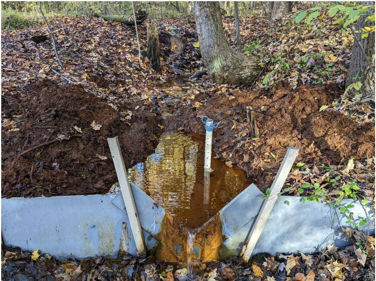
AMD flows through a weir on the southern part of the Friendship Hill property.
