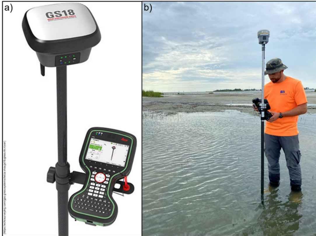
Figure A-1: RTN Rover and Controller/Data Collector Setup – Example of a typical RTN rover and controller/data collector setup (a) and field use of the equipment by EA personnel in a beach environment (b).
