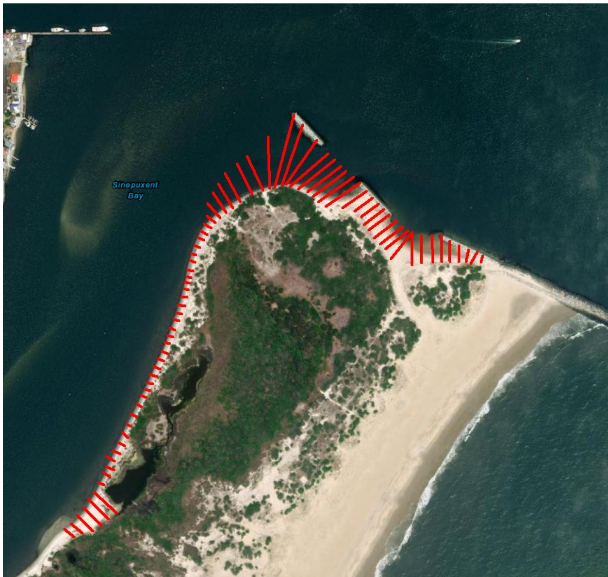
Figure 2: Proposed beach monitoring survey transect layout along the northern shore of ASIS.
