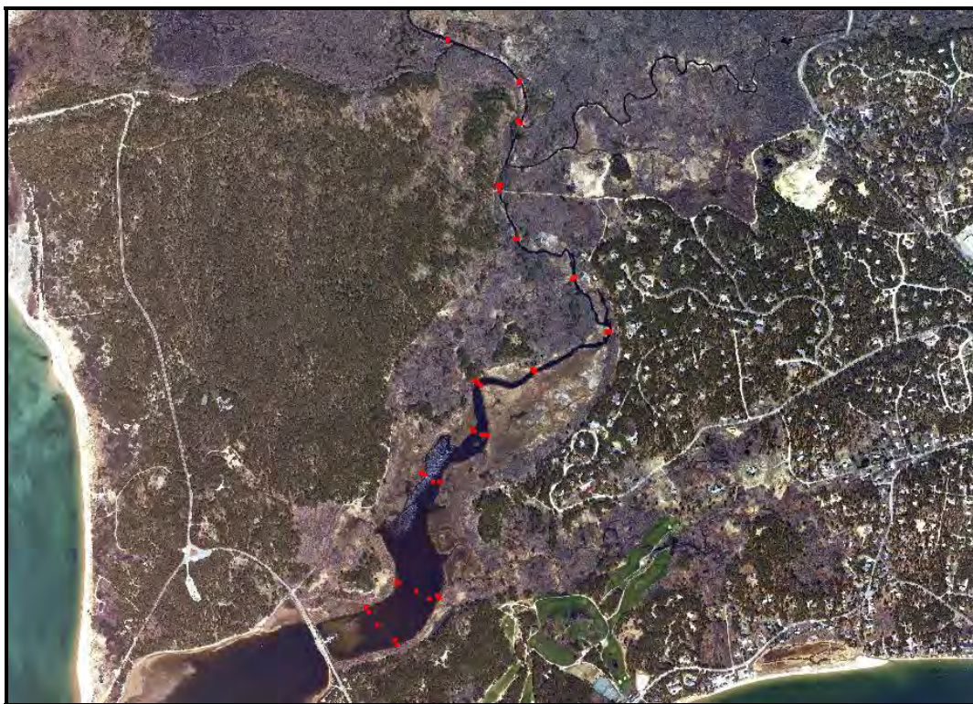
Figure 5-3. Additional RTK-GPS bathymetric cross sections collected by National Park Service in 2008.
