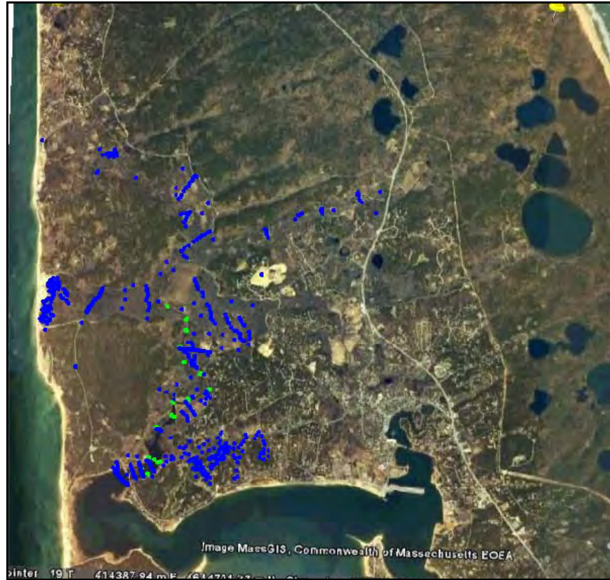
Figure 2-2. Bathymetric data from 1998-1999 NPS total station surveys (blue dots) and 2008 NPS RTK Surveys (green dots) - (background image courtesy of Google Earth).
