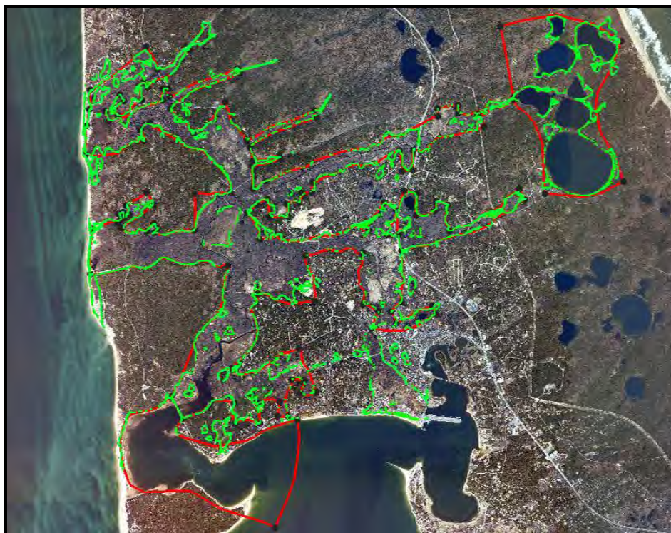
Figure 5-4. 12 foot contour from merged elevation data (green) and block rectangular boundary definition in the physical domain (red).
