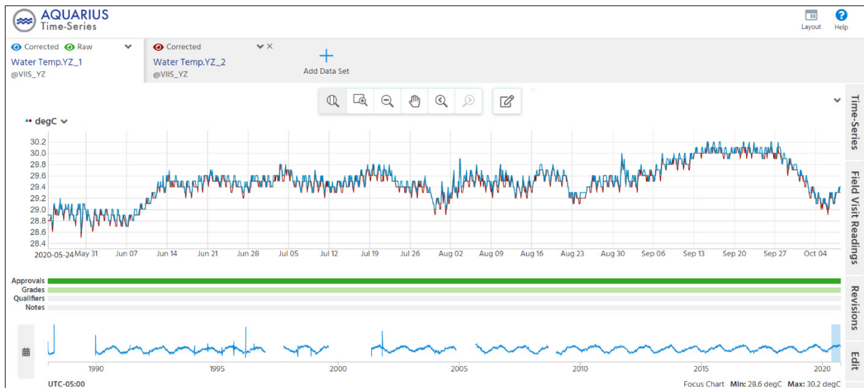
Figure 18. A screenshot of the Data Review Tool with data from two loggers plotted on the same chart. Logger 1 is in blue and logger 2 is in red. This comparison is good for detecting any large disparities between co-located loggers.
