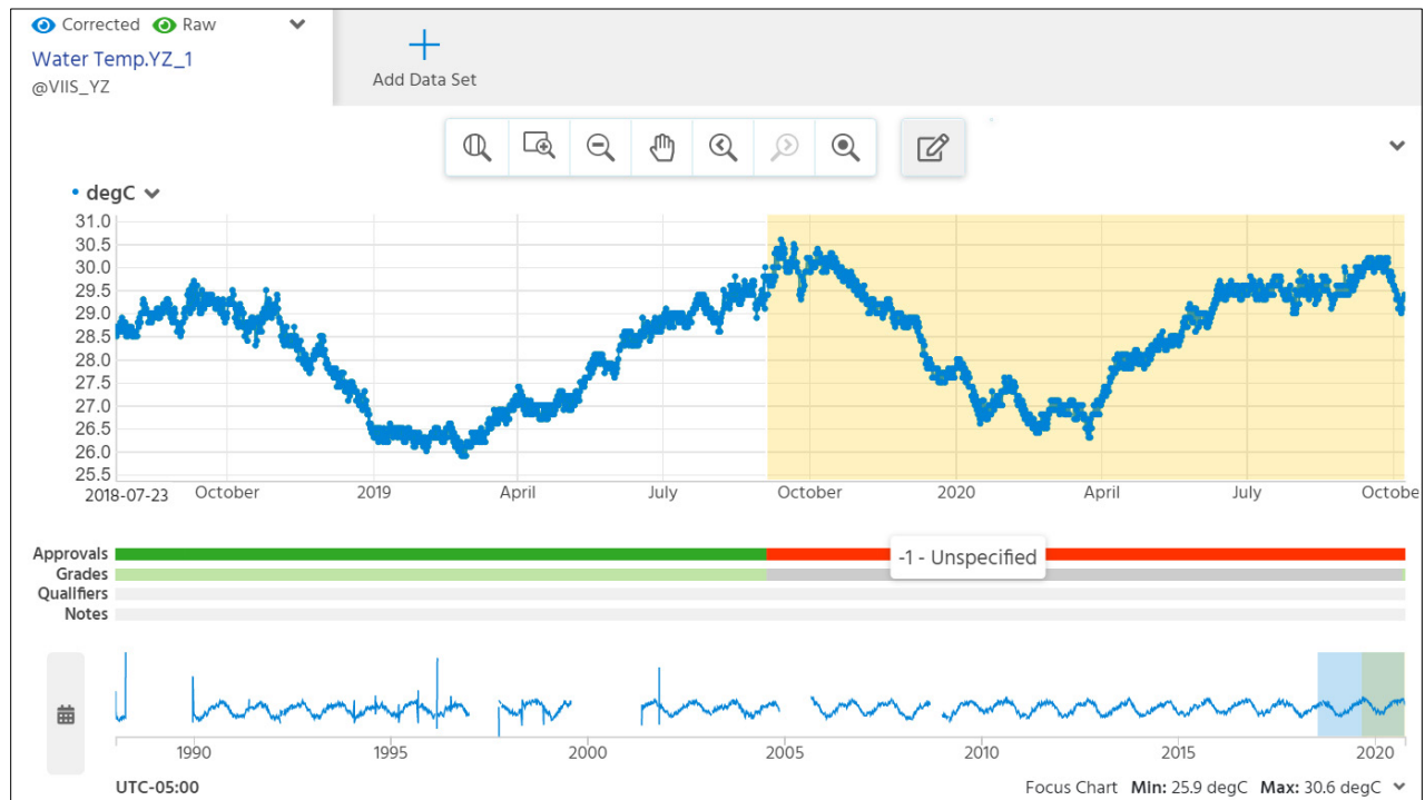
Figure 6. Screenshot showing the Data Review tool. Newly appended data has been selected (highlighted in yellow) by double-clicking the red Approval bar or grey Grade bar in the Metadata Legend.
