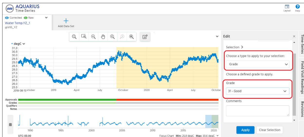
Figure 8. Screenshot showing the Data Review tool with the Edit panel open. Select “Grade” from the drop-down list labeled “Choose a type to apply to your selection”. Apply a grade of “31-Good” by selecting it from the drop-down list labeled “Grade” that appears.
