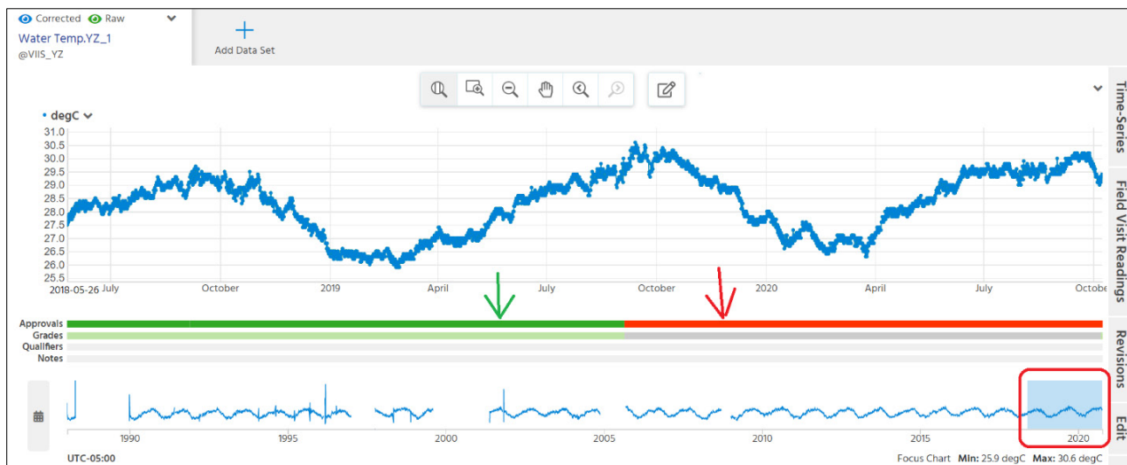
Figure 5. Screenshot showing the Data Review tool. The Focus Chart is the primary user interface. Below this is the Overview Chart showing the full dataset range. The portion of the Overview Chart highlighted in blue is the data that appears in the above Focus Chart. The Metadata Legend, between the two charts, shows the approval and grade settings for various portions of the dataset.
