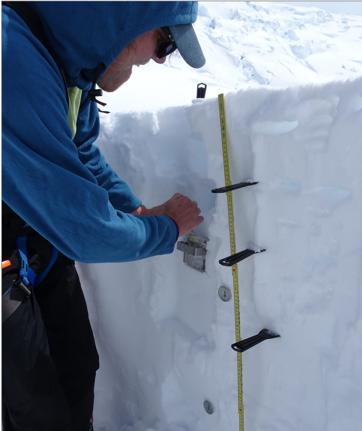
Figure 13. Measuring densities of multiple strata in a snowpit. NPS
