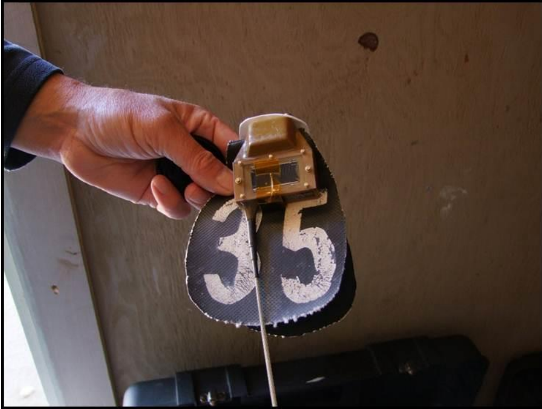
Photo 1. Microwave Telemetry GPS transmitter and wing tag
