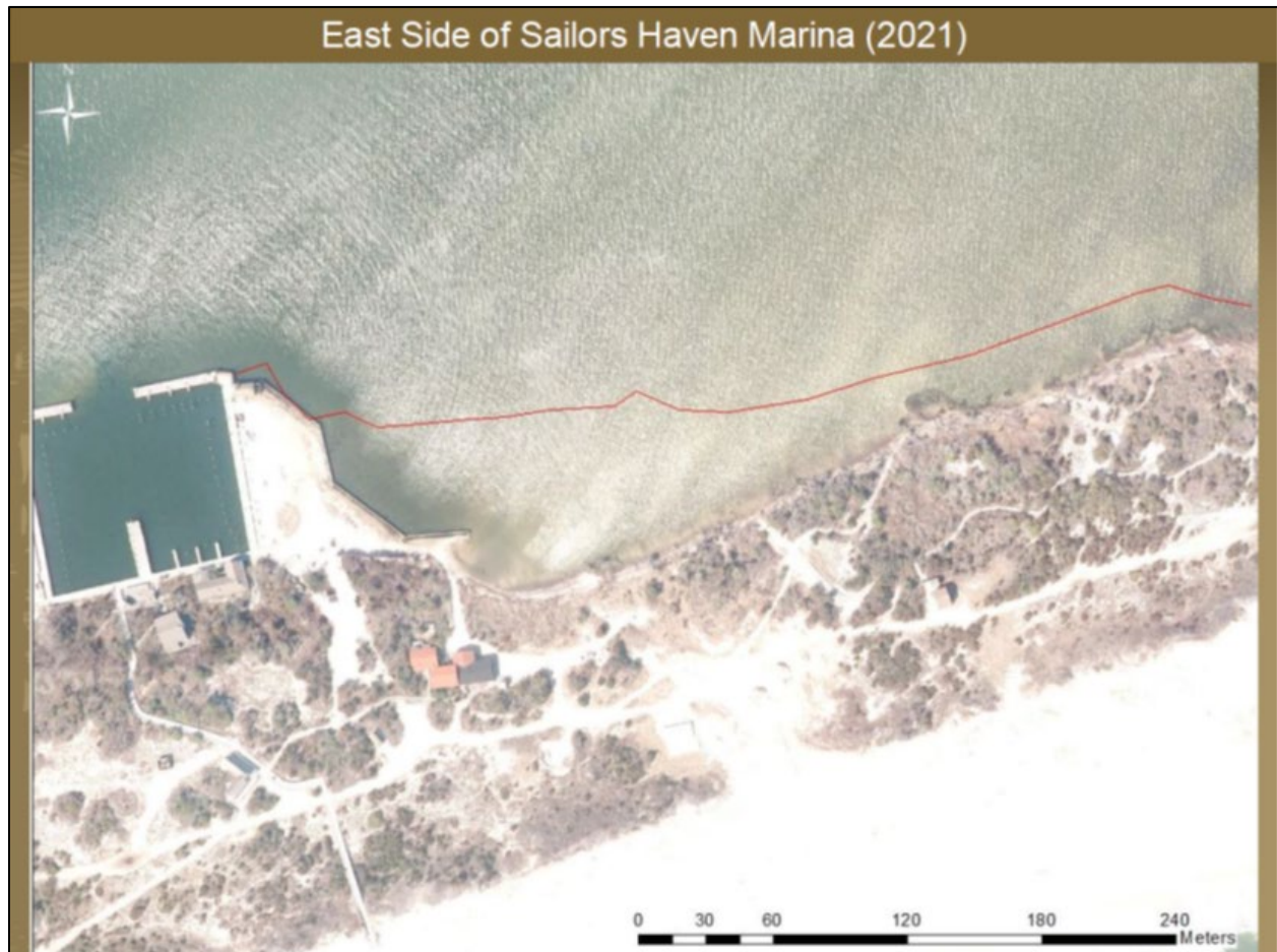
Figure 12 – East Side of Sailors Haven Marina showing approximately 100 feet of shoreline erosion between 1969 (red line) and 2021 imagery (NPS 2021a).
