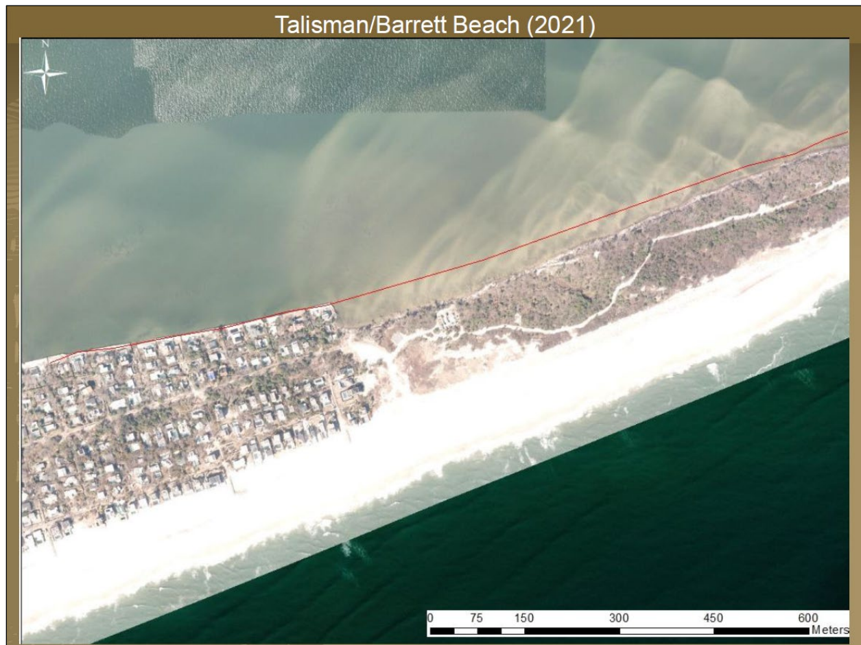
Figure 9 – Talisman showing approximately 30 to 60 feet of shoreline erosion between 1969 (red line) and 2021 imagery (NPS 2021a).
