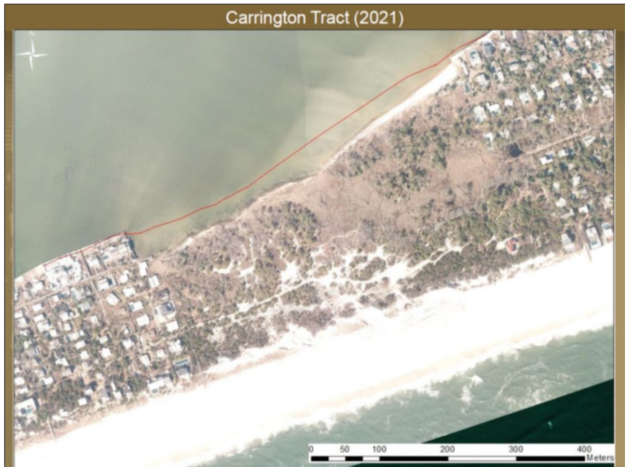
Figure 10 – Carrington Tract showing approximately 165 feet of shoreline erosion between 1969 (red line) and 2021 imagery (NPS 2021a).
