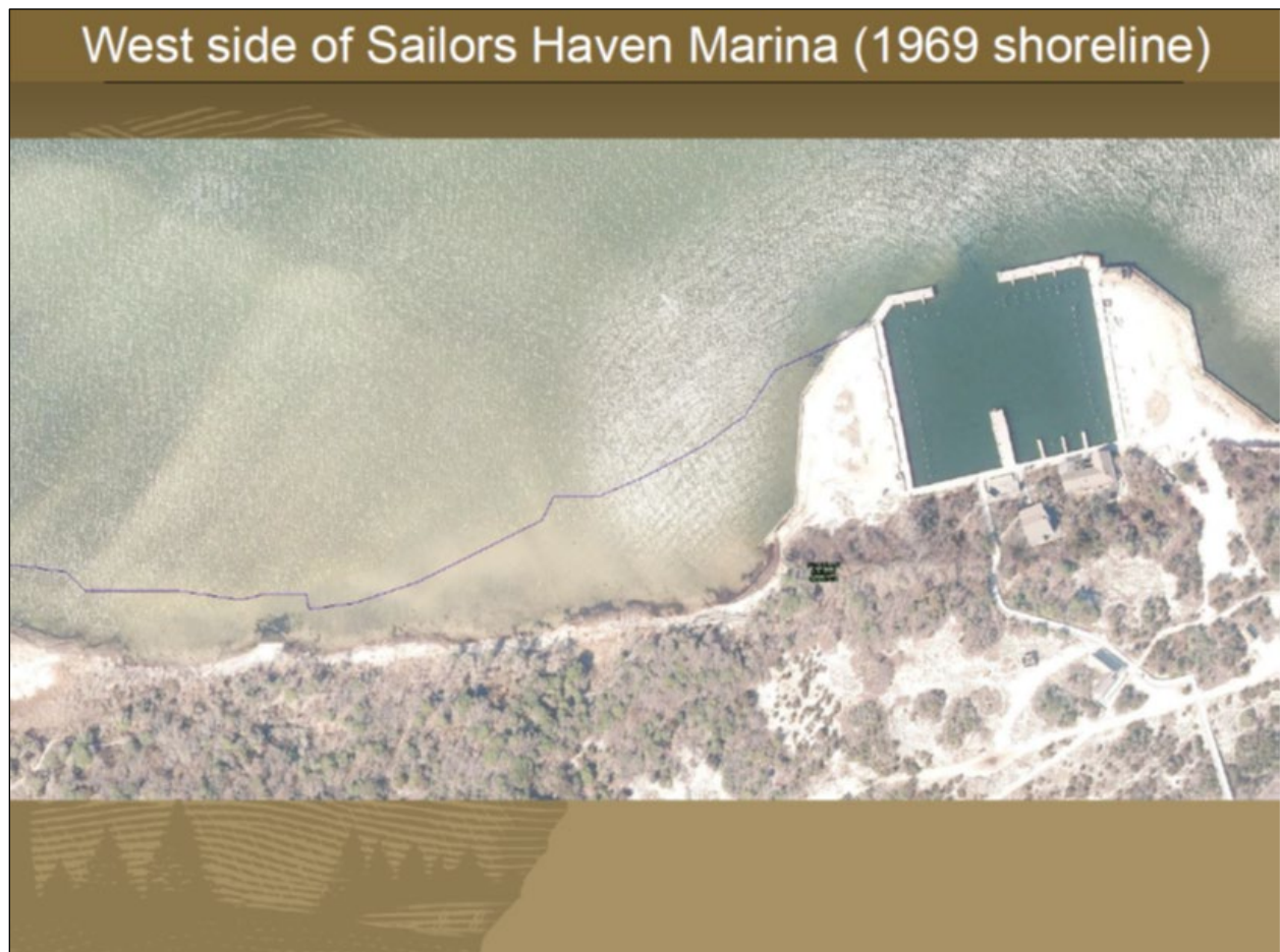
Figure 11 – West Side of Sailors Haven Marina showing approximately 60 feet of shoreline erosion between 1969 (purple line) and 2021 imagery (NPS 2021a).
