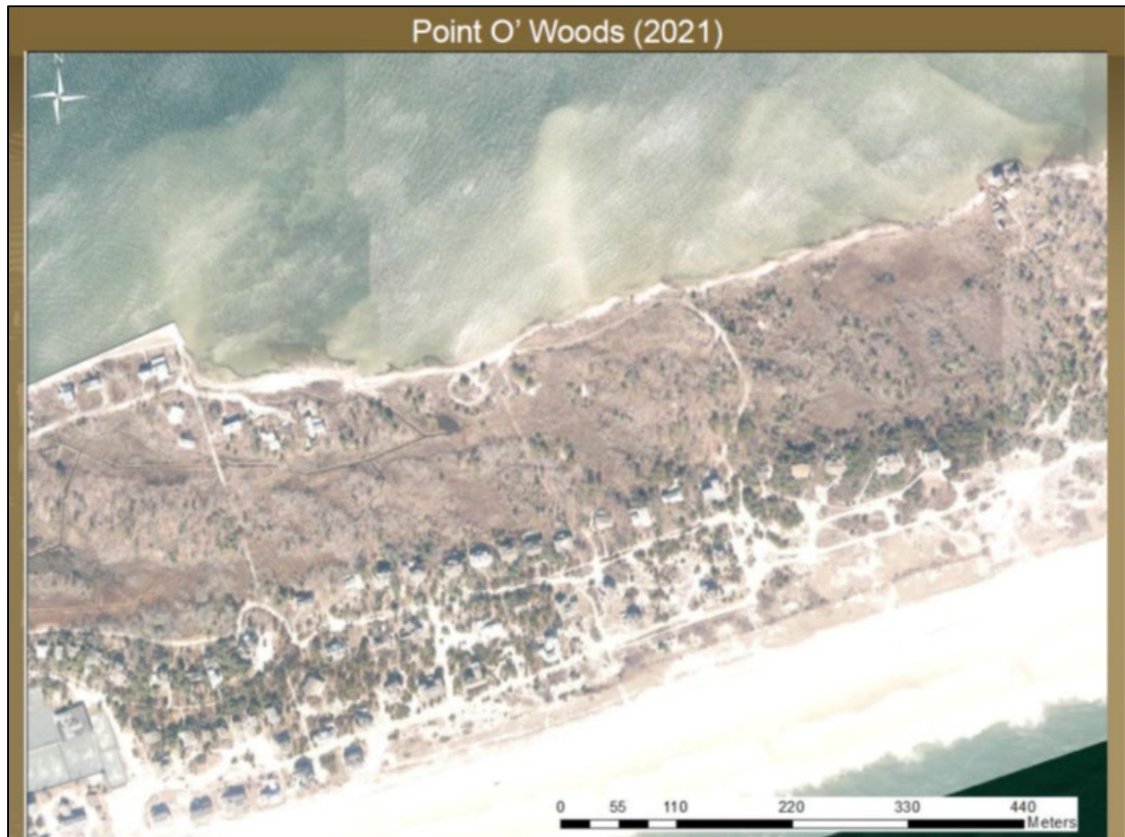
Figure 13 – Aerial image of Point O'Woods showing the 2021 shoreline (NPS 2021a). While aerial imagery from 1969 is not available for this site, assuming it was contiguous with hardened features, the current shoreline would have eroded approximately 50-70 feet since 1969.
