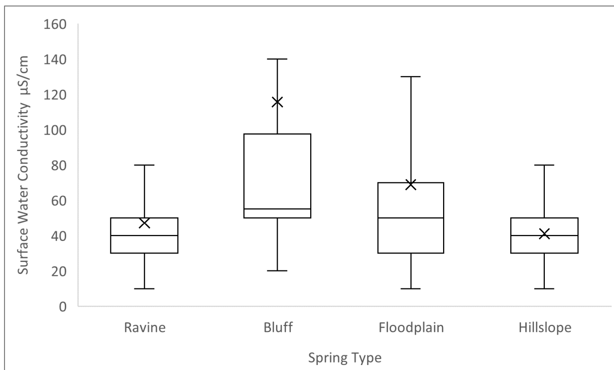
Figure 9. Box plot of conductivity readings from seeps and springs sorted by spring types. Mean for each category is indicated by a cross; the median of each category is the horizontal line within each box. NPS / THOMAS MCCOY-BRUCE
