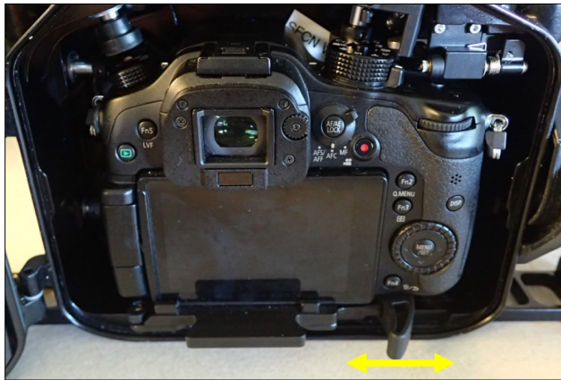
Figure 9. Camera tray lock arm. Movement to the left is “lock” position, to the right is “unlock”.
