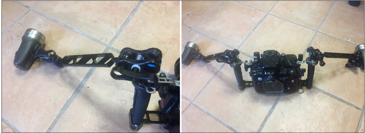
Figure 12. Arrangement of Video light arms and connectors.
