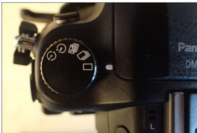
Figure 2. Indicator for single image setting.
