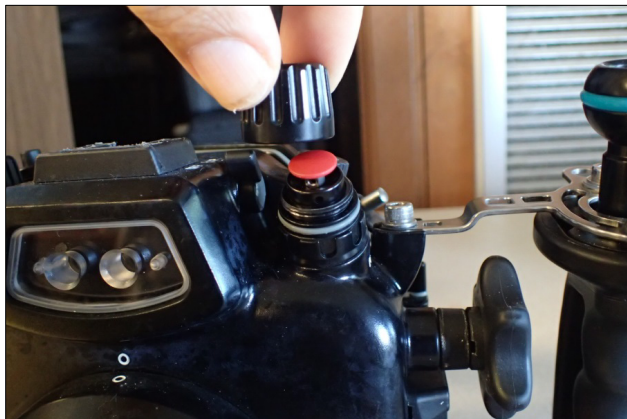
Figure 11. Cap covering vacuum port for leak detection alarm system.
