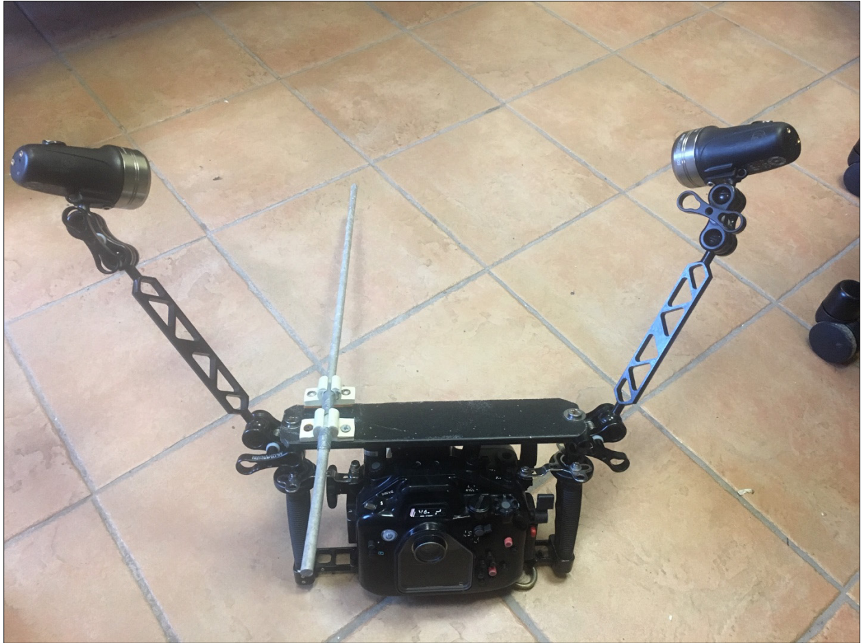
Figure 14. Arrangement of lights and aiming wand.
