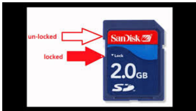
Figure 14. SD card showing the over-write locked and un-locked position.
