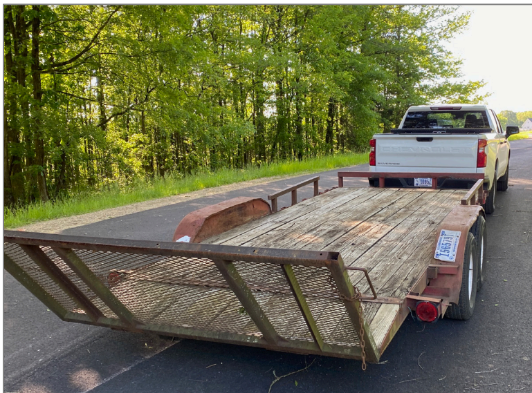
Figure 7. Truck and trailer test vehicle used in passby experiment in NATR on 5/3/23. NPS / KELSEY WHITE
