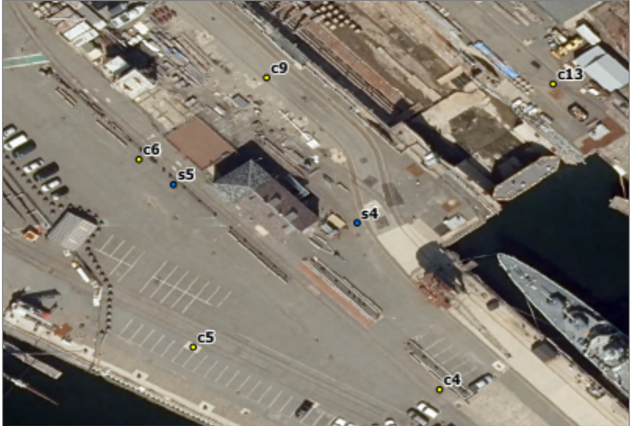
Figure 5. Aerial view of the Charlestown Navy Yard, Boston National Historical Park, over Building 10 and Pier 1 depicting two scan locations and four control points. Scan s4 used control points c9 and c4 for resection, and scan s5 used control points c5 and c6 for resection.
