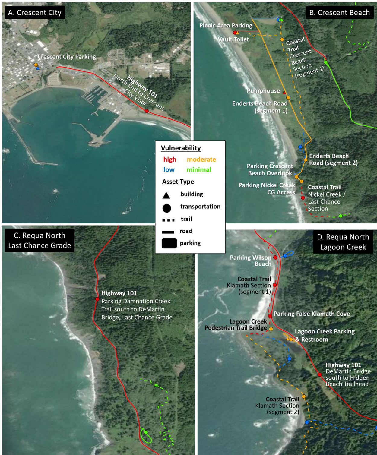
Figure 3. REDW vulnerability results summary for the A) Crescent City, B) Crescent Beach, C) Requa North - Last Chance Grade, and D) Requa North - Lagoon Creek areas. Only high and moderate vulnerability assets are labeled. Background is 2022 ESRI world imagery.
