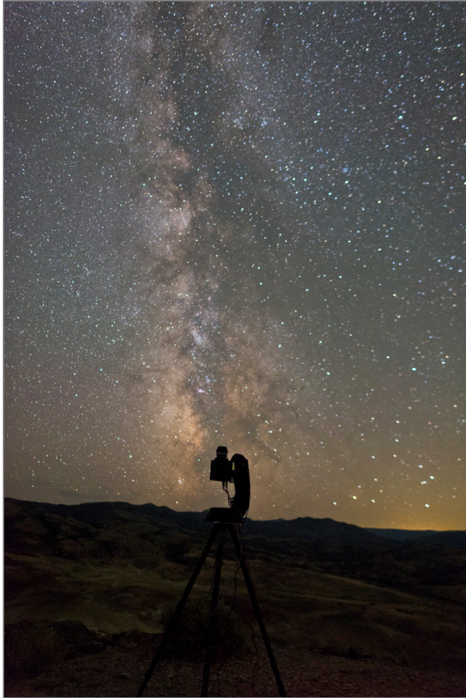
Figure 2. A typical National Park Service Night Skies Program camera system consists of a commercial lens, a V-band filter, and a CCD camera. The camera system is mounted on a motorized mount, hooked up to external batteries, and controlled by a computer.
