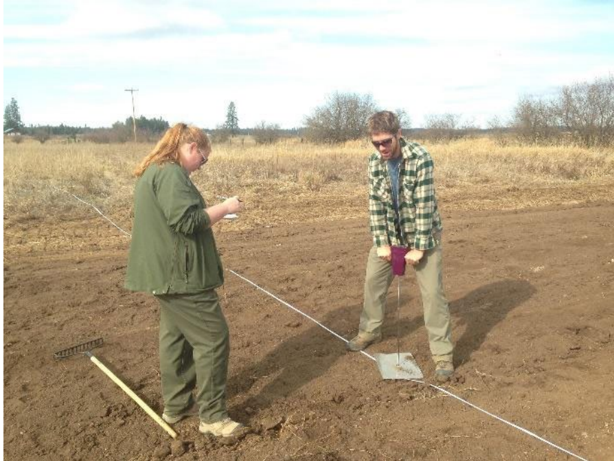
Figure A7. Measuring soil density profiles along a transect in the filled zone. Surveyors shown are Derek Schook and Katy Matthews.
