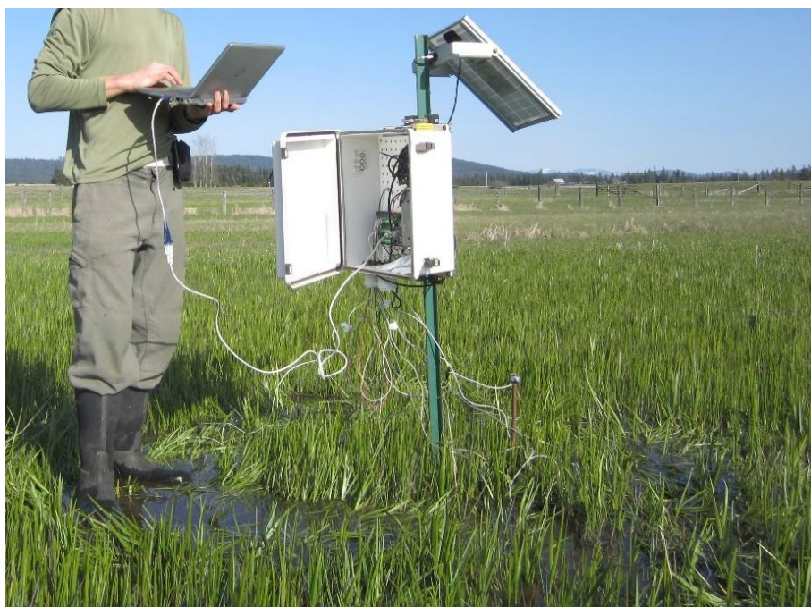
Figure A2. A station that was used to measure the oxidation-reduction potential of the near-surface soil during the growing seasons of 2012 and 2013.
