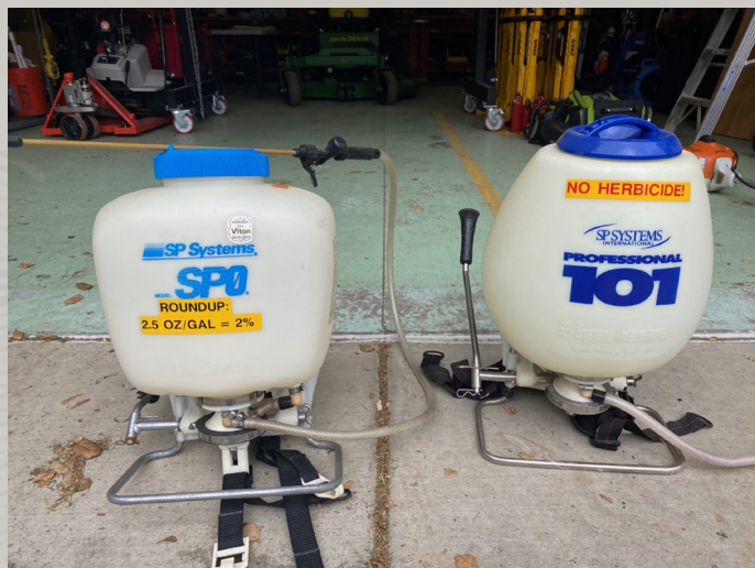
Clearly labelling sprayers for distinct uses prevents cross-contamination. (NPS)
