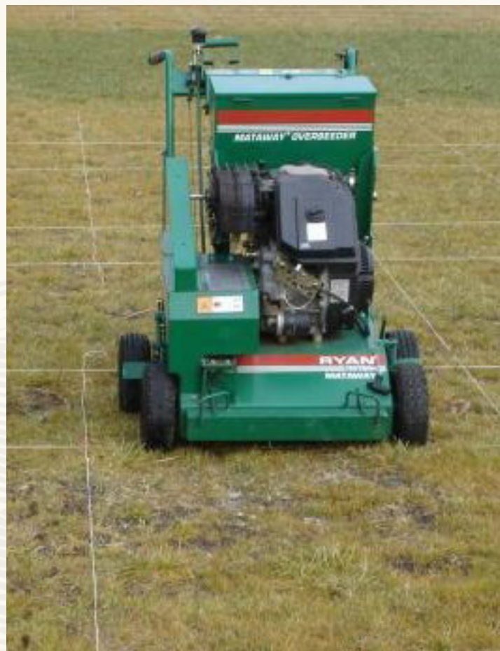
Slit seeders can be used to sow seed. (NC State Extension)
