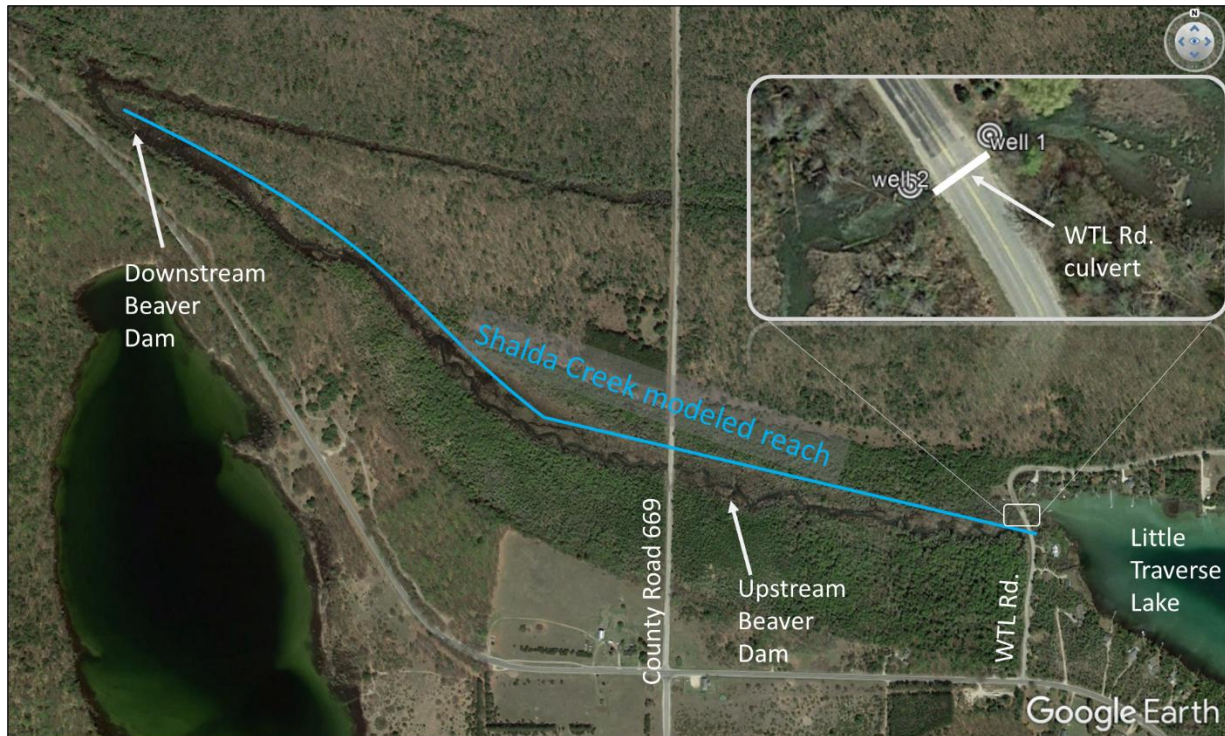
Figure 1. The Shalda Creek modeled reach (blue). Inset map at top-right shows West Traverse Lake Rd, its small arch culvert (white line), and wells 1 and 2. Flow is from right to left. Google Earth image 2018.
