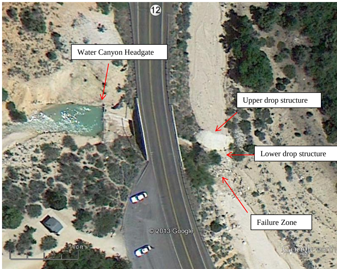
Figure 1 - Google Earth image of the site at the confluence of the Paria River and Water Canyon. The Paria River channel runs north-south and Water Canyon enters from the west. Note the drop structure adjacent to the bridge crossing, all of the visible water is being diverted into an underground pipe, but on a regular basis, the system is “flushed” of sediment by diverting the imported water directly into the Paria River.
