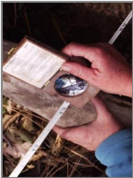
Figure SOP 23.2. Using a spherical densiometer to measure riparian canopy closure.
