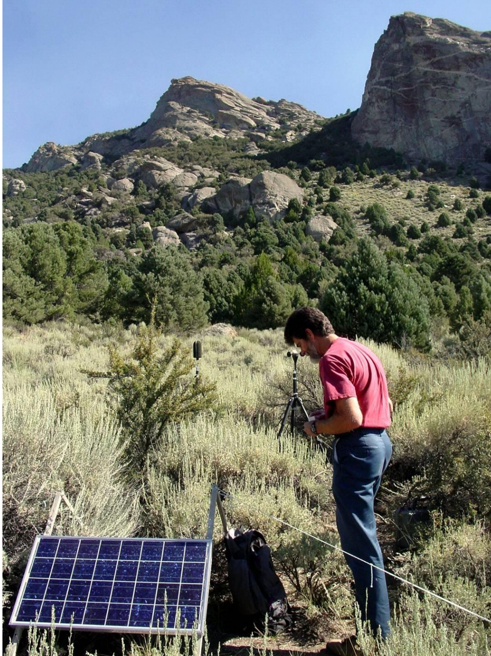
Figure 1. An example of an acoustical monitoring set-up at CIRO002, Geo-Watt Trail, in the park's natural area. Solar panel is seen in foreground. The microphone (left) and anemometer (right) are seen in the background.
