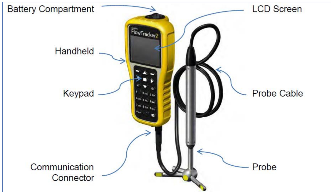
Figure SOP 24.1. FlowTracker2 handheld unit and its various components.
