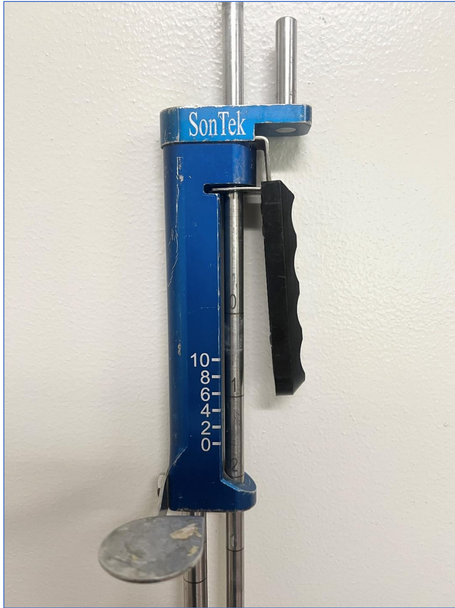
Figure SOP 24.7. The top of the wading rod set to a depth of 0.16 m. When setting the depth, the number on the thin pole indicates the digit in the tenths place, and should align with the number on the handle, which indicates the hundredths place. For a depth of 0.16 m as shown above the 1 on the thin pole aligns with the 6 on the handle. If the depth were 0.26 m, the user would squeeze the handle and raise the thin pole such that the 2 on the pole would align with the 6 on the handle.
