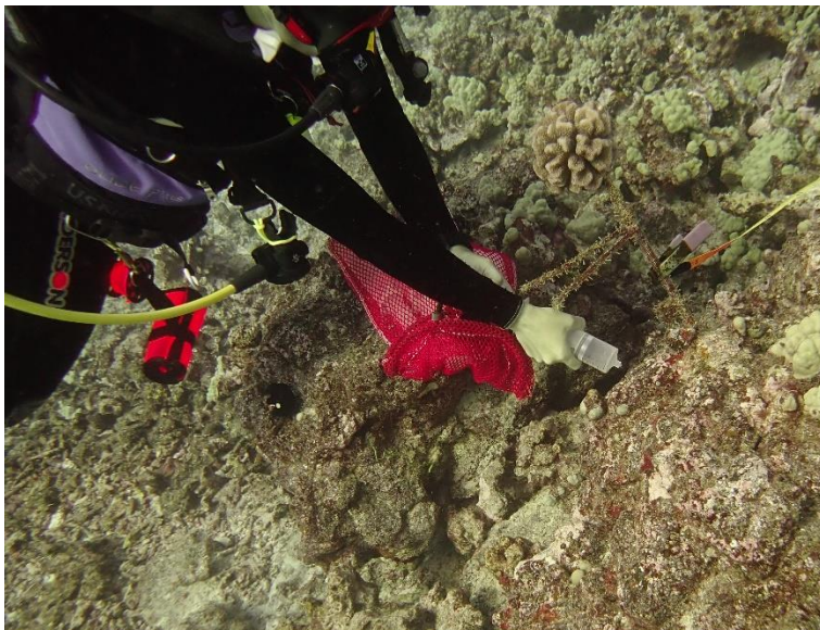
Figure SOP 11.3. Collecting a water sample underwater with a syringe.
