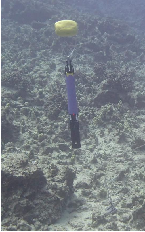
Figure SOP 11.2. Sonde deployed underwater.
