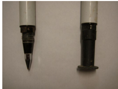
Figure 8. Options for the bottom of prism poles. The point on the left is used for control points, top of headpins, and well shots while the flat foot is on the right is used for all other shots. Leveling rods only have a flat foot.
