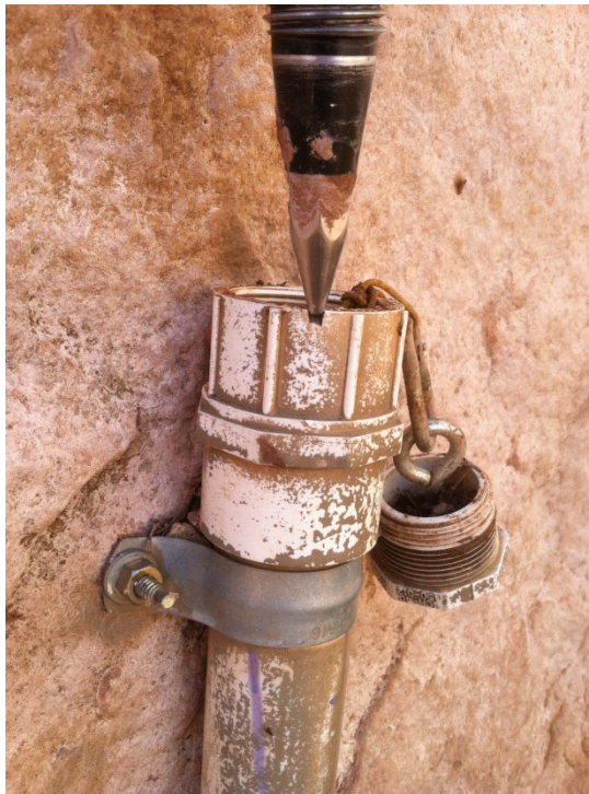
NABR. The rod point in the measuring notch. This was how the “TOC-NOTCH” shot was taken in 2015.
