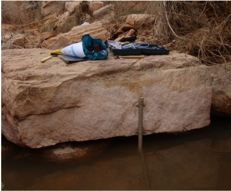
Figure 8. PVC casing instream installation at Natural Bridges National Monument.
