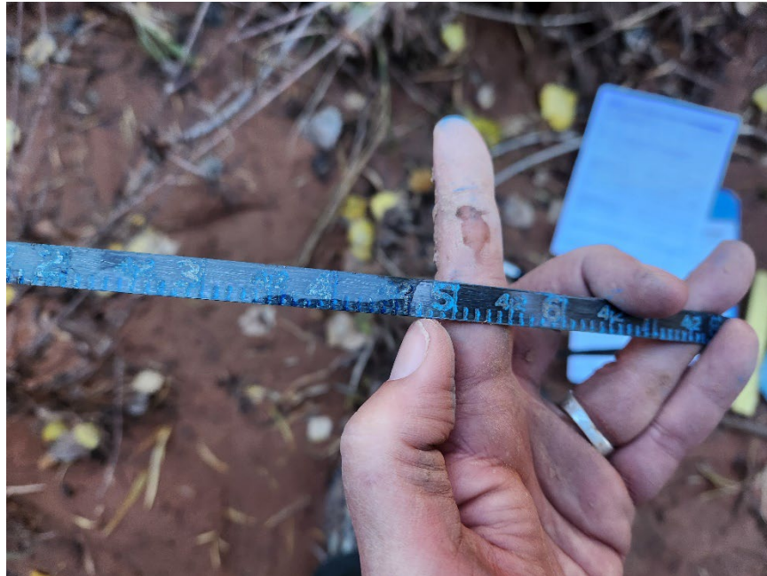
Figure 11. Example of depth to water measurements using steel tape. The wetted chalk mark reads 42.46 ft.
