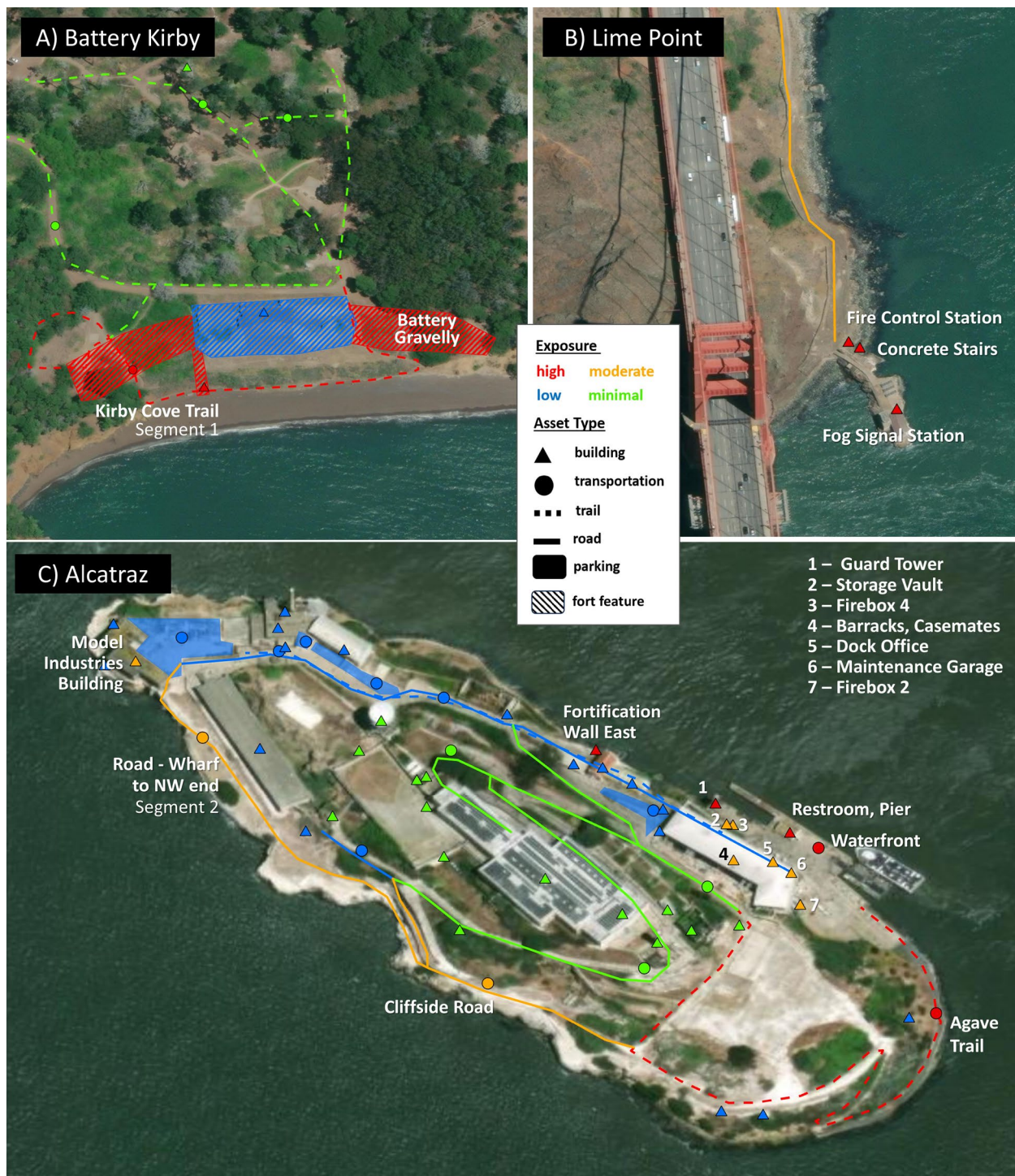
Figure 4. GOGA exposure results summary for the A) Battery Kirby, B) Lime Point, and C) Alcatraz areas. Only high and moderate exposure assets are labeled. Background is 2022 ESRI Streaming World Imagery.
