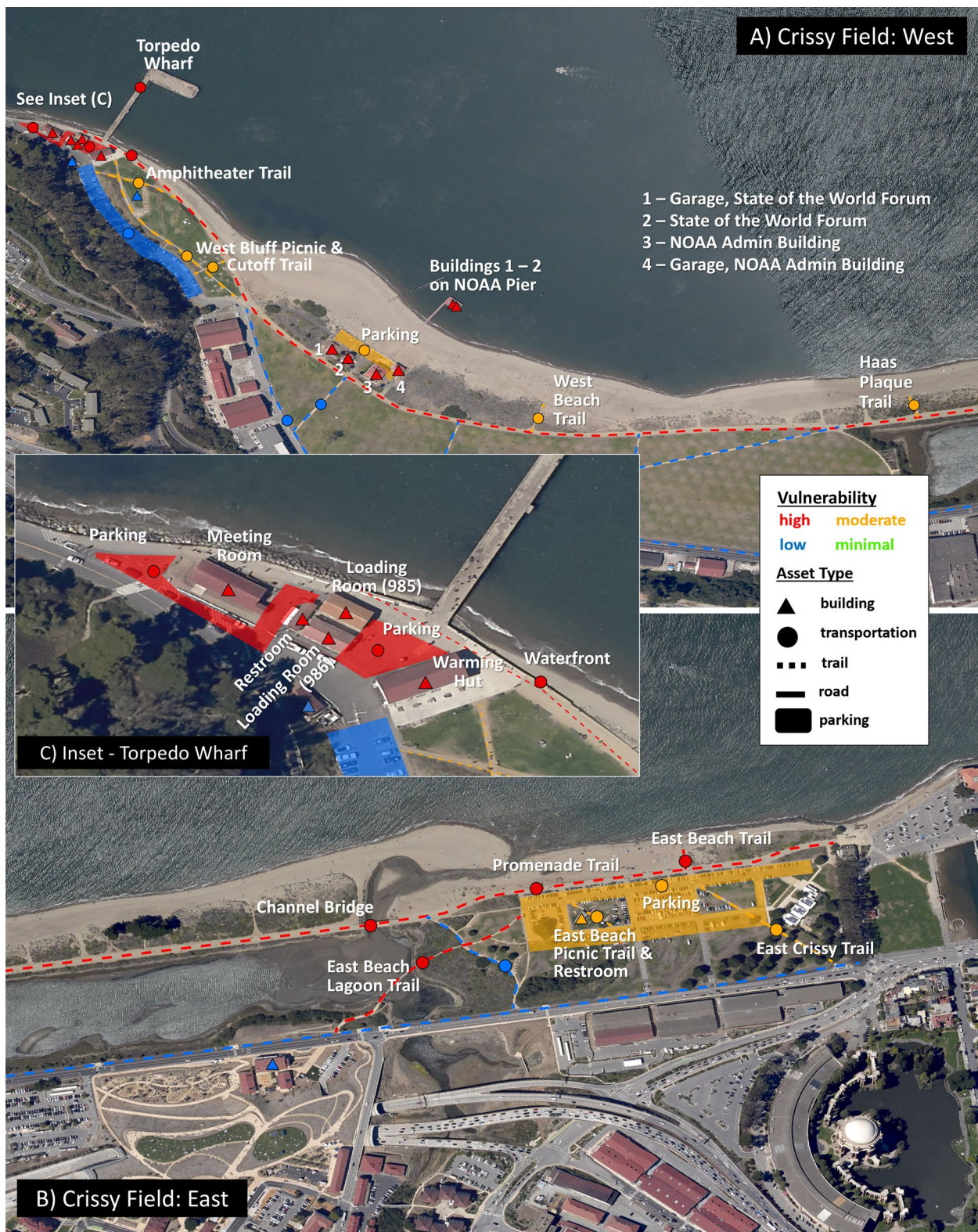
Figure 18. PRSF vulnerability results summary for the A) Crissy Field: West, B) Crissy Field: East, and C) Inset - Torpedo Wharf areas. Only high and moderate vulnerability assets are labeled. Background is NOAA NGS 2022 imagery (NGS 2025a).
