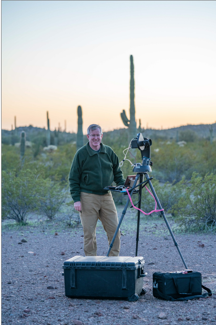
Figure 2. The NPS Night Skies camera system setup in Organ Pipe Cactus National Monument. A typical National Park Service Night Skies Program camera system consists of a commercial lens, a V-band filter, and a CCD camera. The camera system is mounted on a motorized mount, hooked up to external batteries, and controlled by a computer.
