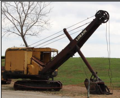
Lorain Tracked Excavator (ca. 1954)
