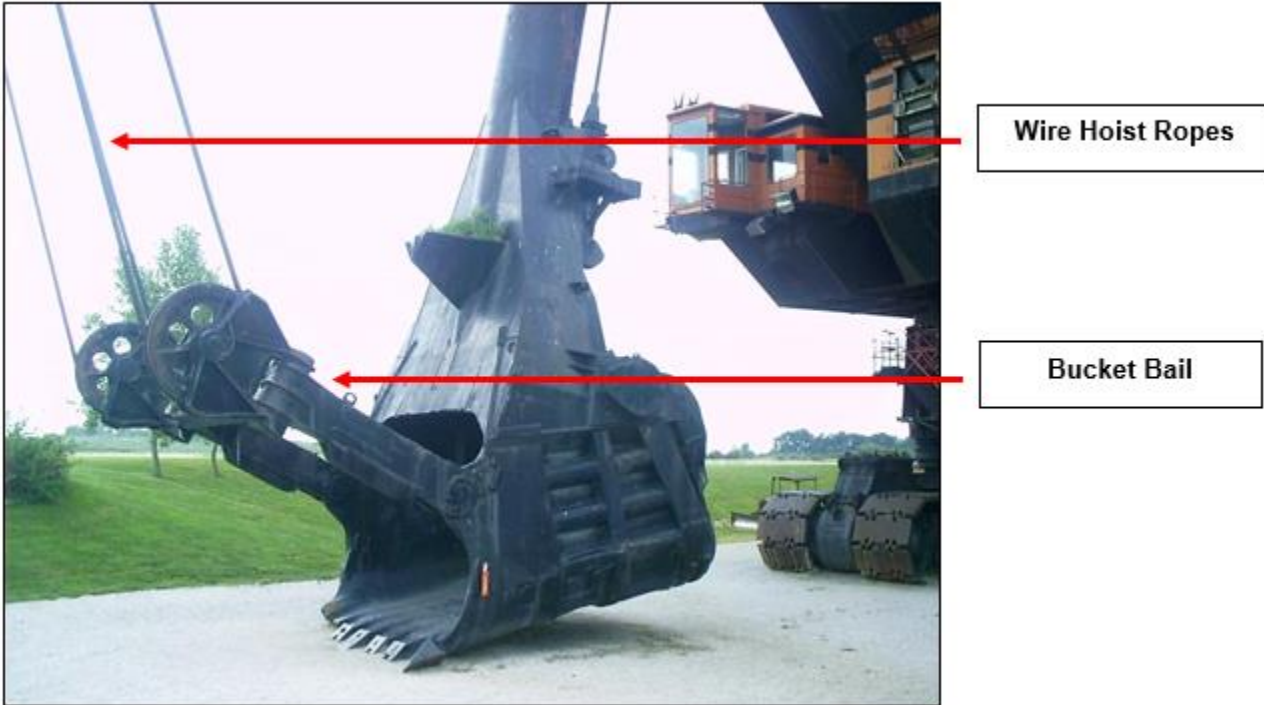
Figure 4: Bucket and hoist ropes today.
