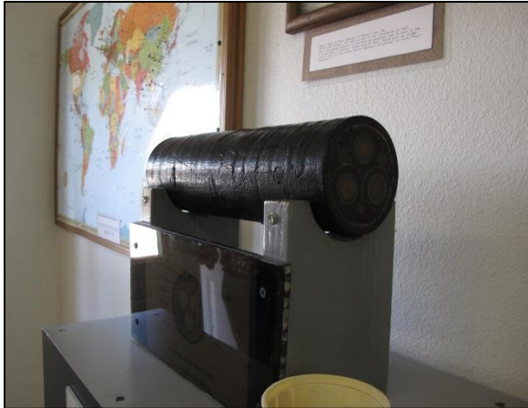
Figure 14: Sample of the power cable
