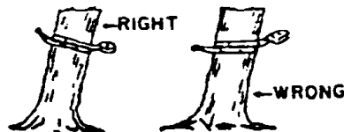
The tape must be at right angles to the lean of the tree.
