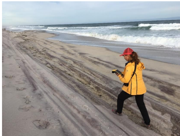
Figure 4. Using a Trimble Geo7x to map the spring tides by walking along the high-water line.
