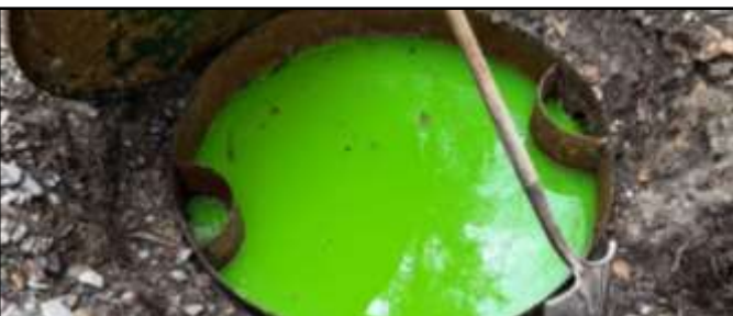
Left: Bright green tracing dye used for testing wastewater systems (NPS Photo). Right: Tracing dye traveling underground shown in a wastewater system (NPS Photo).
