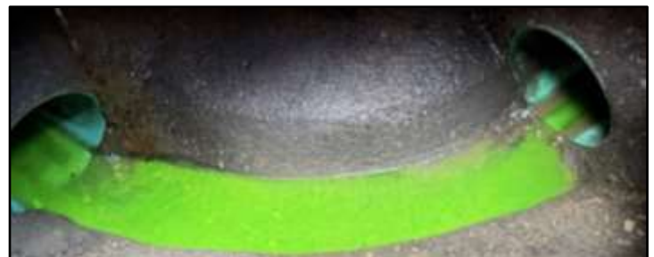
Left: Bright green tracing dye used for testing wastewater systems (NPS Photo). Right: Tracing dye traveling underground shown in a wastewater system (NPS Photo).
