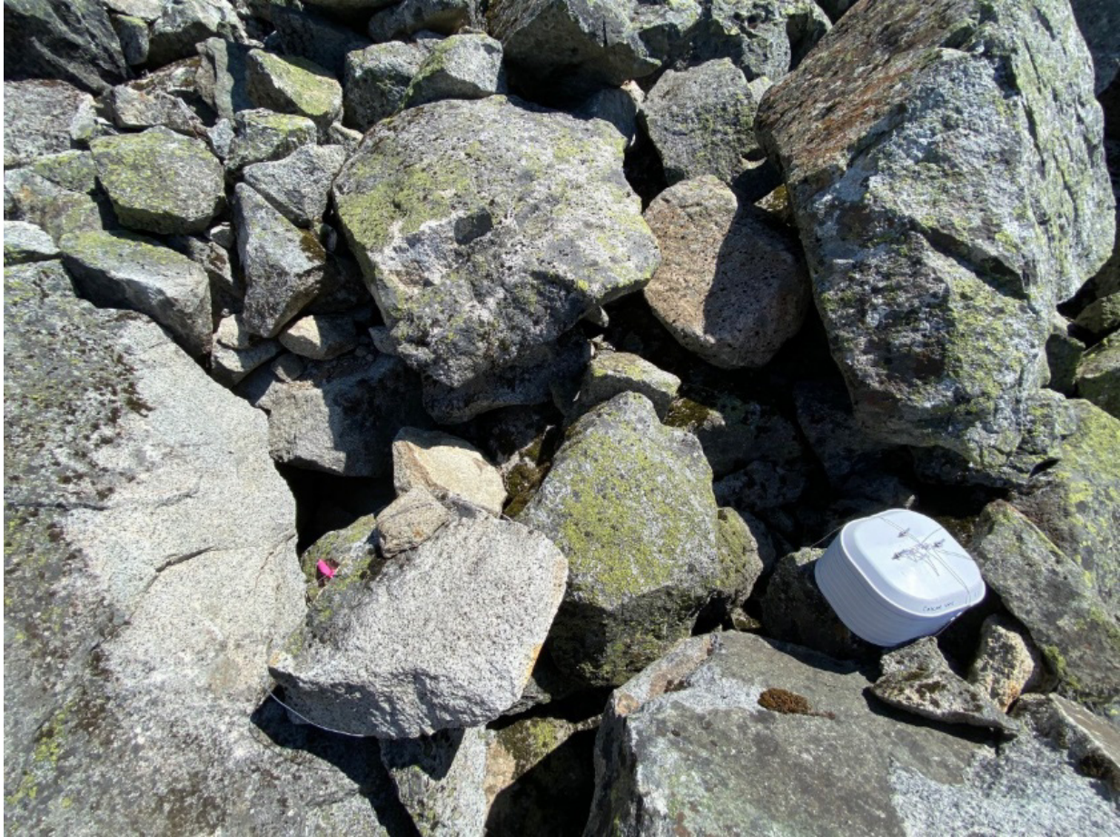
Fig 2. Datalogger station in situ, with above ground solar radiation shield anchored to a surface boulder (right) and the entrance to its paired subsurface datalogger marked with pink flagging (left).
