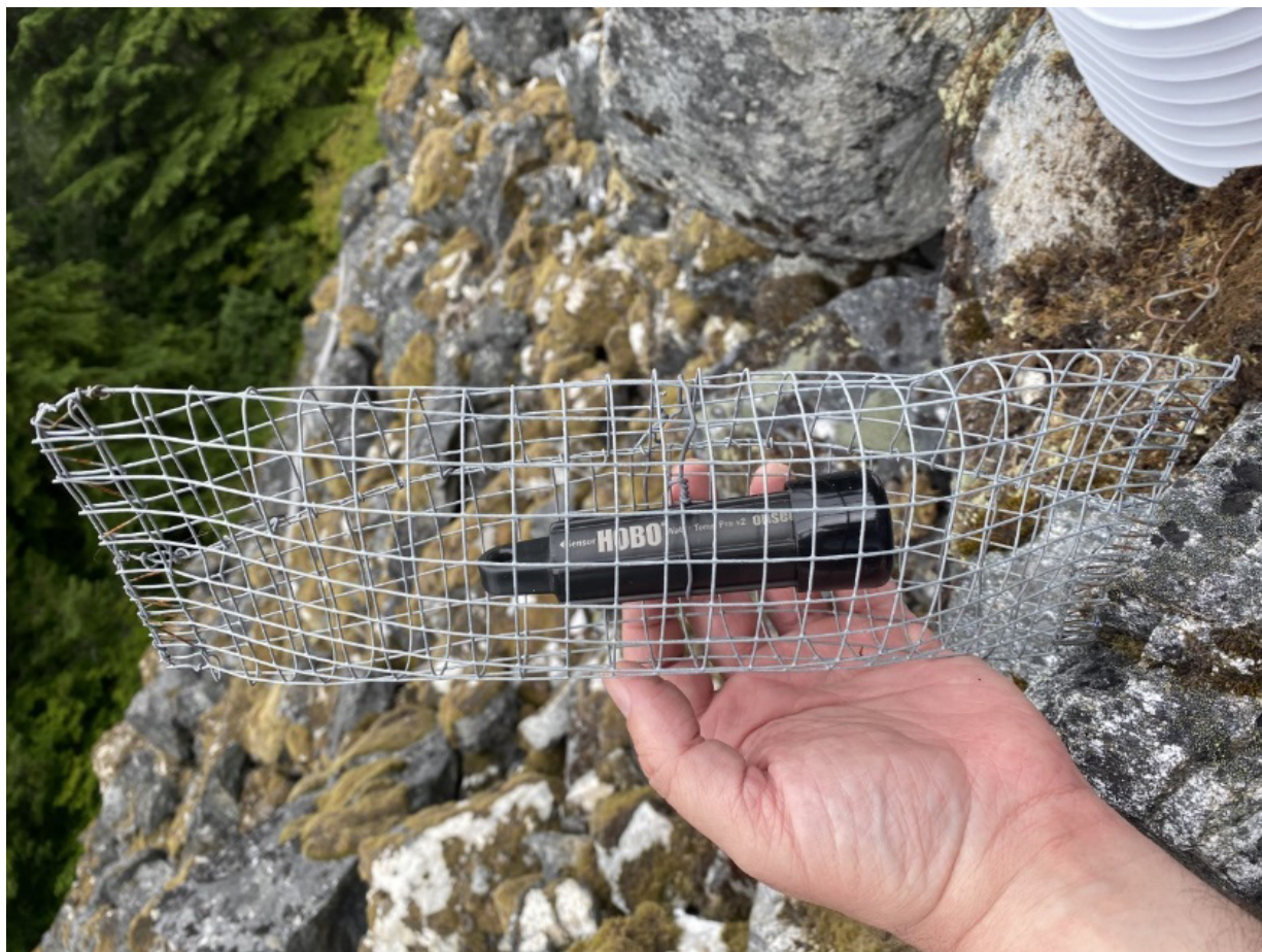
Fig. 1. Subsurface datalogger suspended in its protective cage.
