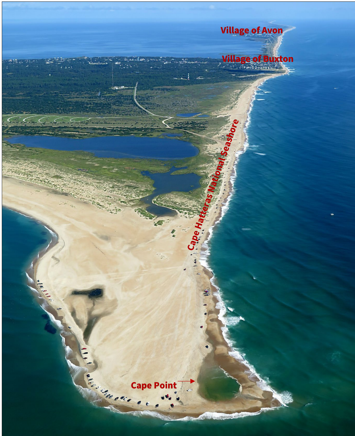
FIGURE 2.1. Aerial photo taken on 10 September 2014 showing sand movement from north to south and a sand deposit at Cape Point. Sand also accumulates from the west at Cape Point under prevailing winds and waves from the southwest. [Source: CSE]
