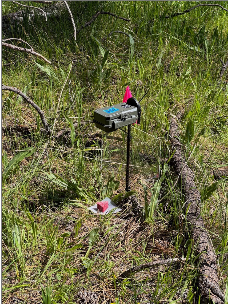
Figure 3. The chew block and camera trap setup. Chew blocks were placed on a white plastic plate, with or without a camera. Cameras were placed at a subset of chew block stations where they were attached to a rebar stake fixed into the ground, ~12–18 inches above the ground, with the lens pointed downward directly at the chew block. A clear plexiglass plate was affixed to the rebar stake to funnel animals into the camera view and temporarily hold back vegetation from interfering with the camera view.
