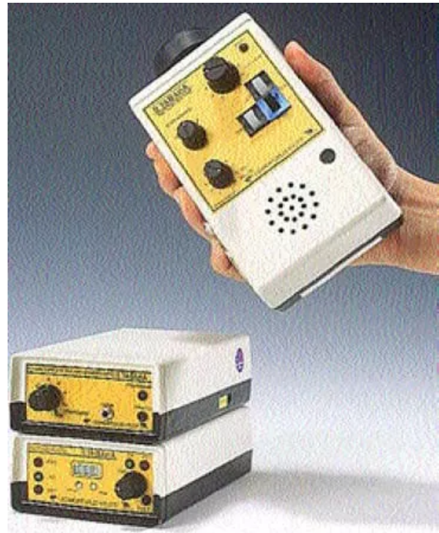
The Ana Bat II Detector System was used to record ultrasonic echolocation calls of bats at Pinnacles National Park. Titley Electronics, Australia
