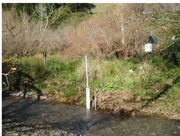
A typical streamflow monitoring setup, including gauges to manually measure water depth and peak flow depth (center left), a transducer to automatically measure and record water level (center right), a rain gauge (back left), and a solar powered, weather-protected datalogger (back right).
