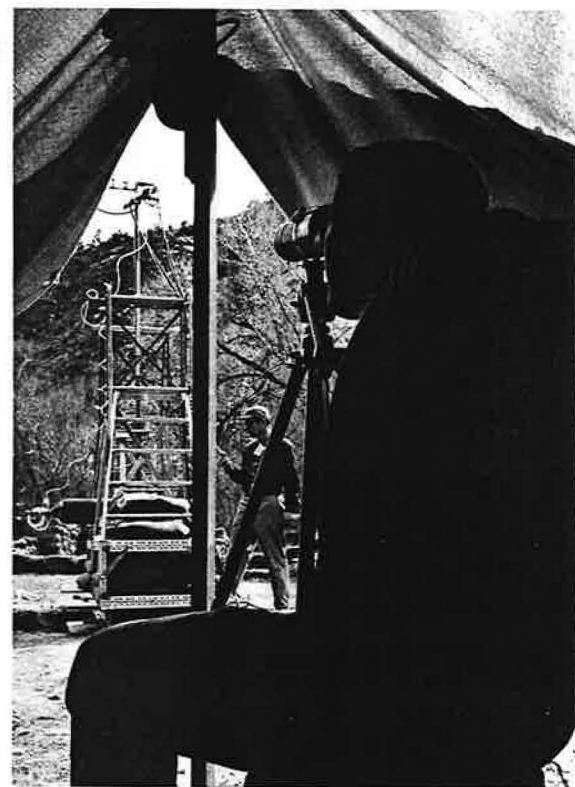
Olivas checks melting rate by viewing measuring stick on stem of subterrene through telescope.
