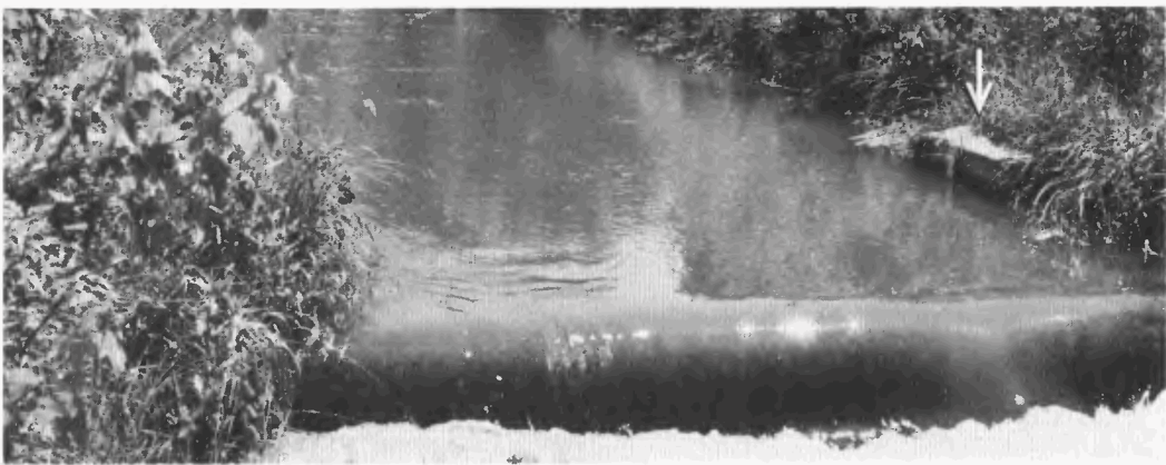
FIGURE 11.—Channel of North Branch Rock Creek near Rockville. Intake for automatic pumping suspended-sediment sampler is located on concrete pier (arrow) (view from downstream).
