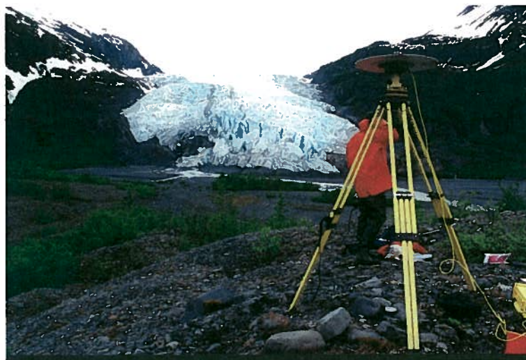
Figure 3. Trimble 4000SSi GPS receiver set up over control NPS13A.
