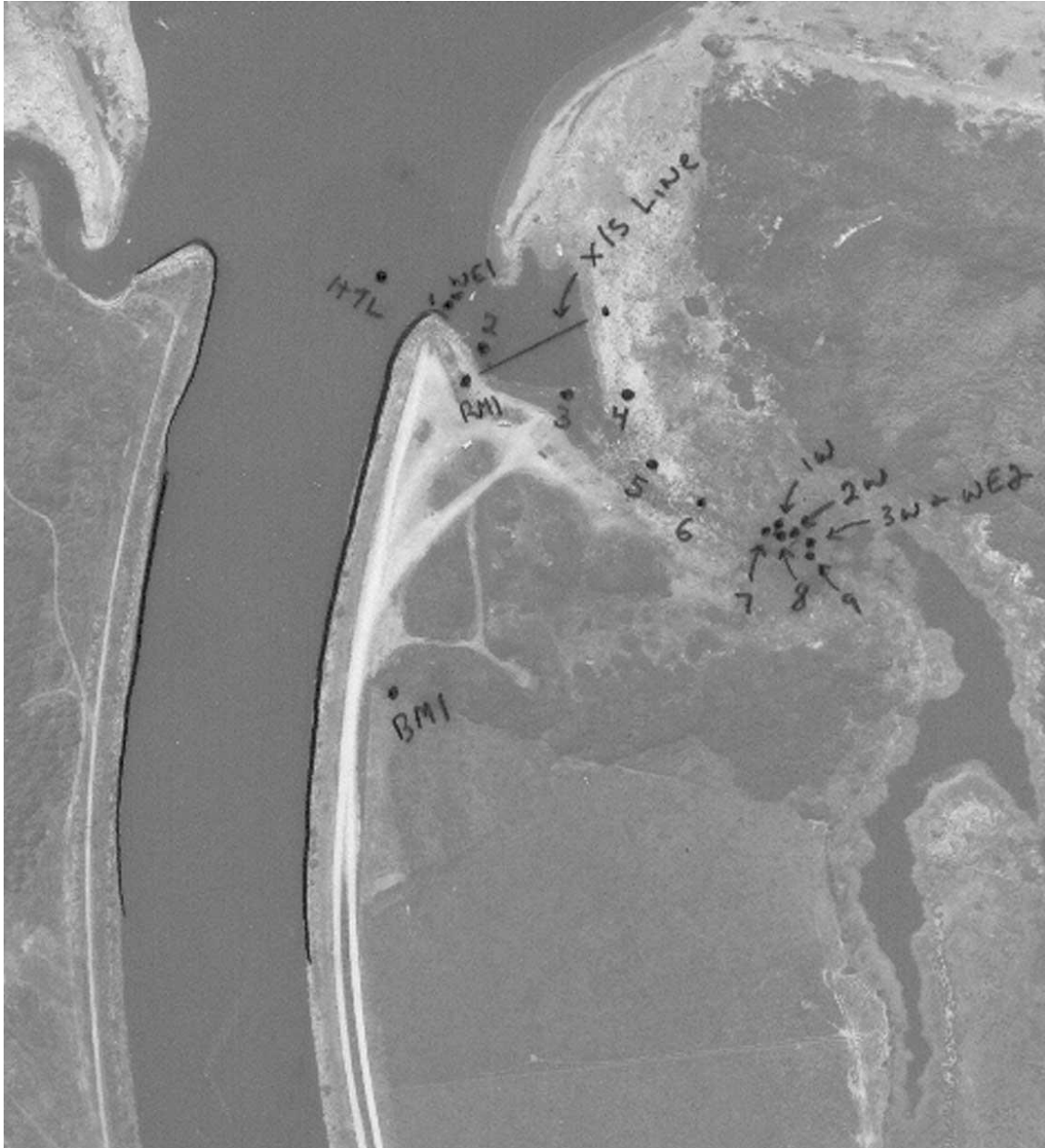
Figure 7. Survey points from May 30, 2001 longitudinal and cross-section survey of the North Slough Channel. The longitudinal survey started at the end of the north levee (point #1) and extended into the North Slough (point #8). Points 1W – 3W and #9 were on top of the accumulated driftwood in the remnant channel. The cross section (X/S Line) went west from benchmark RM1. The High Tide Line (HTL) at 3.25-ft Mean Sea Level elevation was located in the embayment of the Redwood Creek Estuary. The aerial photo is an older one and at the time of the survey, the area was dry except for the small outlet channel.
