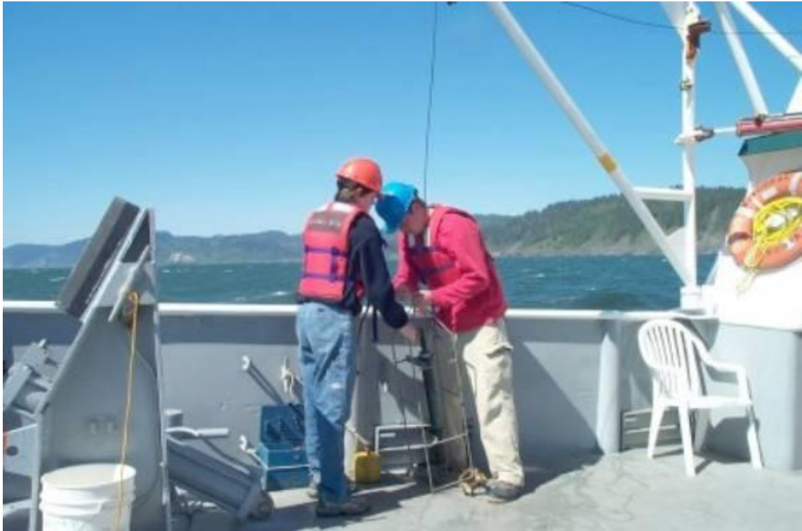
Preparing the CTD. We lowered this device at various locations offshore to search for the surface plume.
