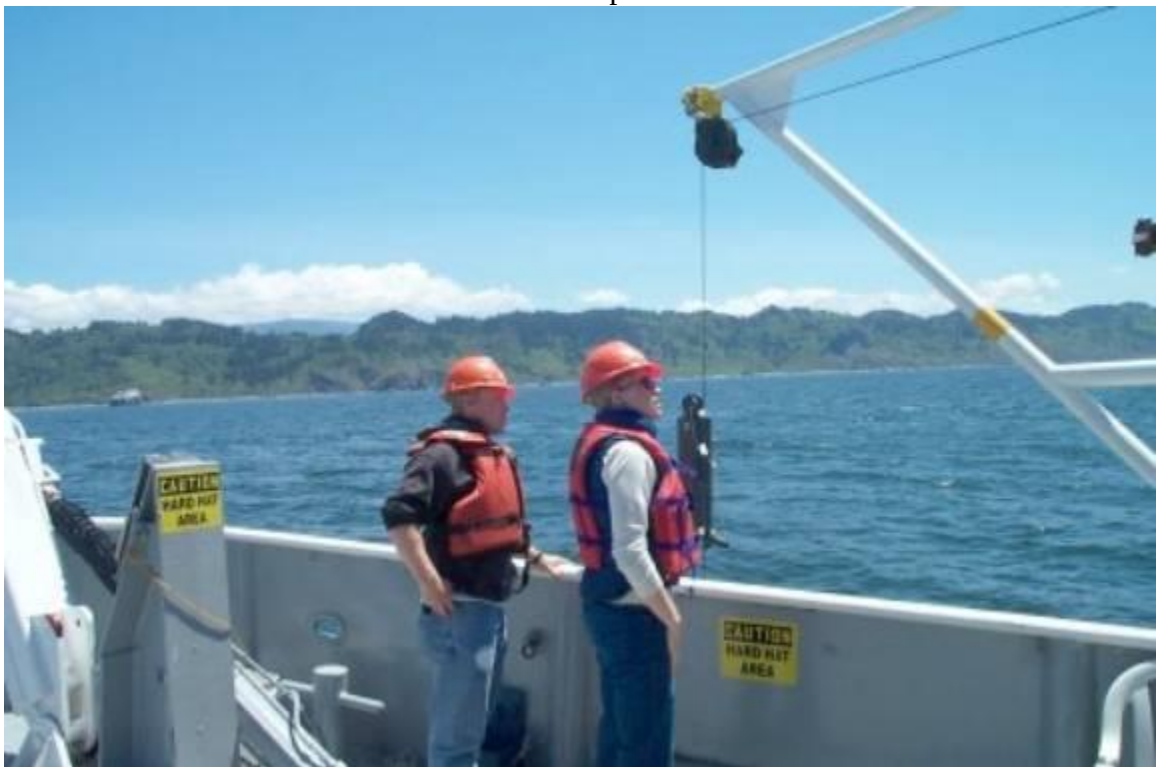
Preparing the CTD. We lowered this device at various locations offshore to search for the surface plume.
