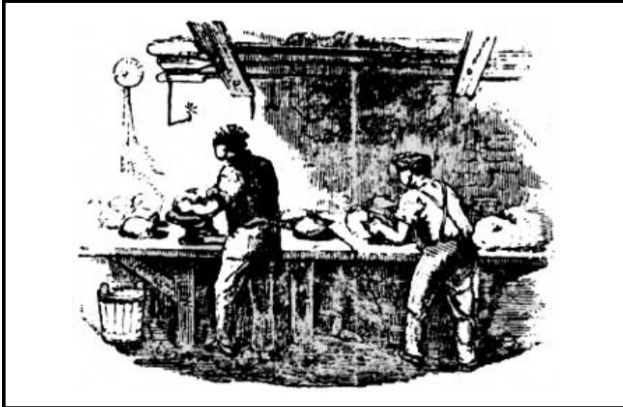
Figure 13. "Scaling off" in an English bakery, c. 1854. The dough removed from the kneading trough sits on the table at the extreme right. The man on the right is cutting the dough into loaf-size pieces which are being weighed by the man on the left. Note shape of bucket under table. Peels are stored on overhead racks. (From Tomlinson, op. cit. , I, 181.)
