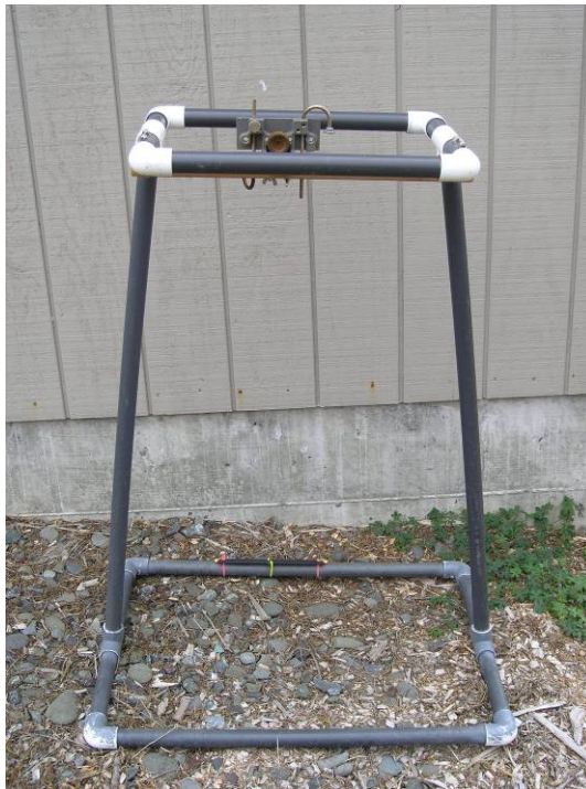
Figure 14. PVC photo framer for photographing permanent 50 x 75 cm plots. A camera (not shown here) was mounted to the top brackets to ensure accurate replicate size.
