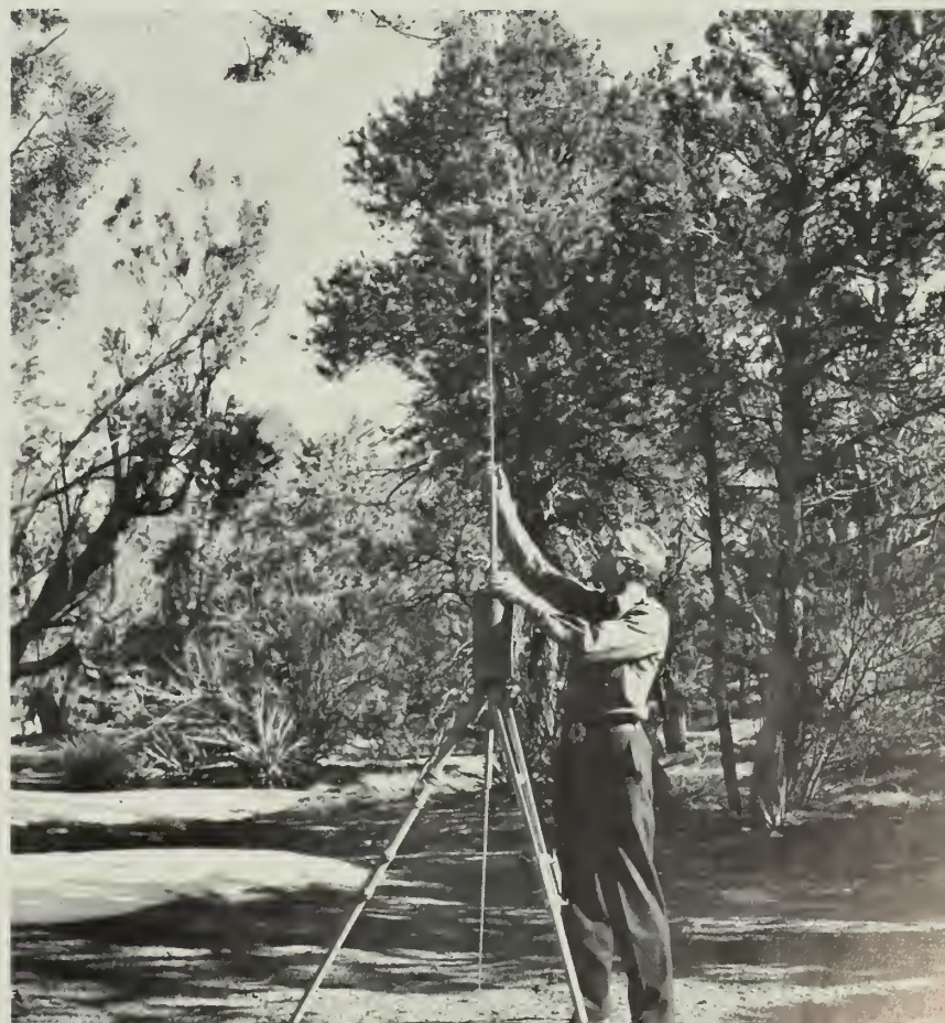
Figure 4—Transmitter and radio direction finder.
