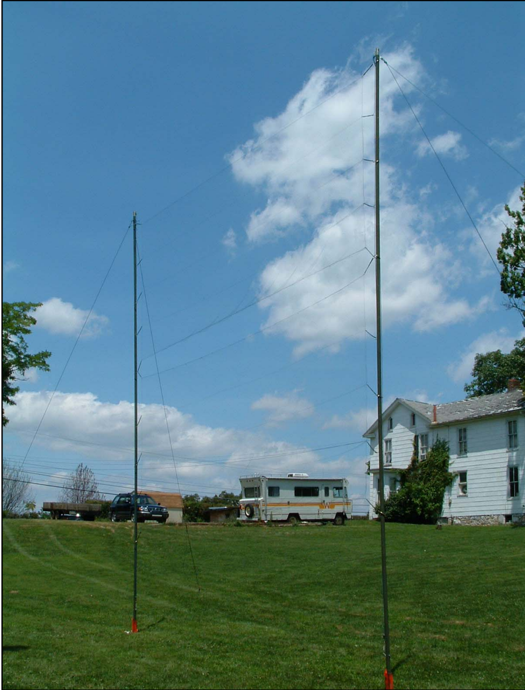
Figure 3. Example of a 9 m high elevated/canopy system erected with three 6 m wide nets attached. This is similar to how the system would be set up at a predetermined mist-netting site.
