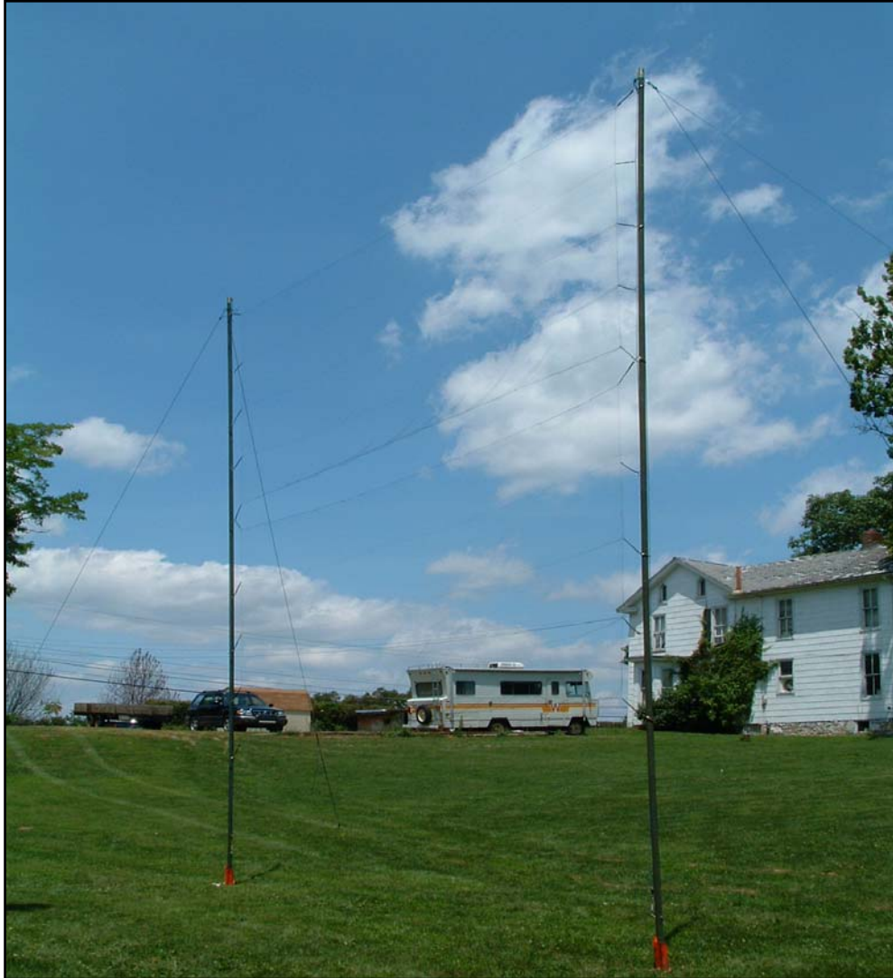
Figure 3. Example of a 9 m high elevated/canopy system erected with three 6 m wide nets attached. This is similar to how the system was set up at a predetermined mist-netting site.
