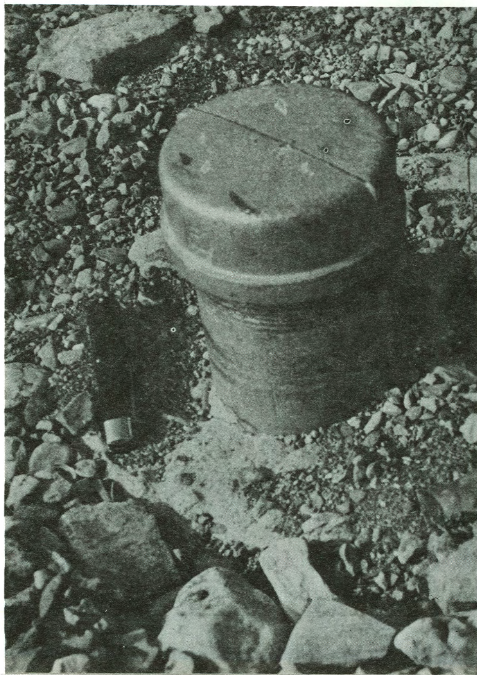
Figure 11. Close-up of upper end of soil moisture tube as installed in channel at upper Ropes Draw Site showing cast-iron sleeve added to prevent washout.
