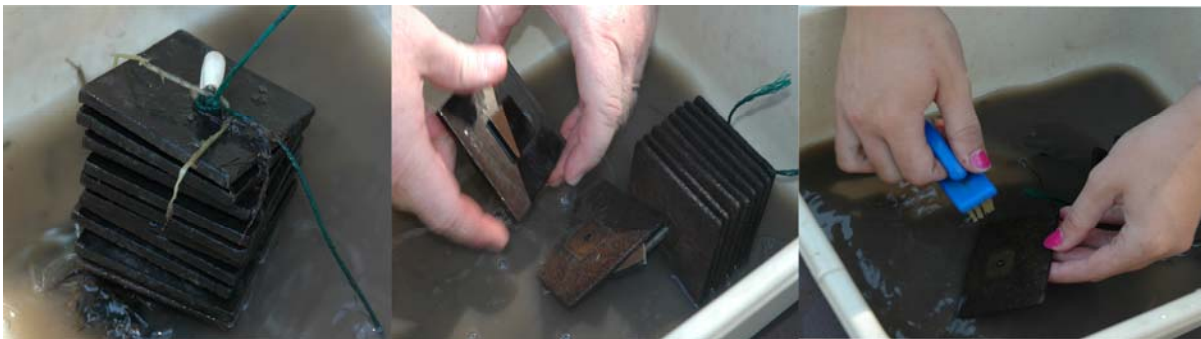
Figure 9. Procedure for removing attached invertebrates from individual Hester-Dendy plates.
