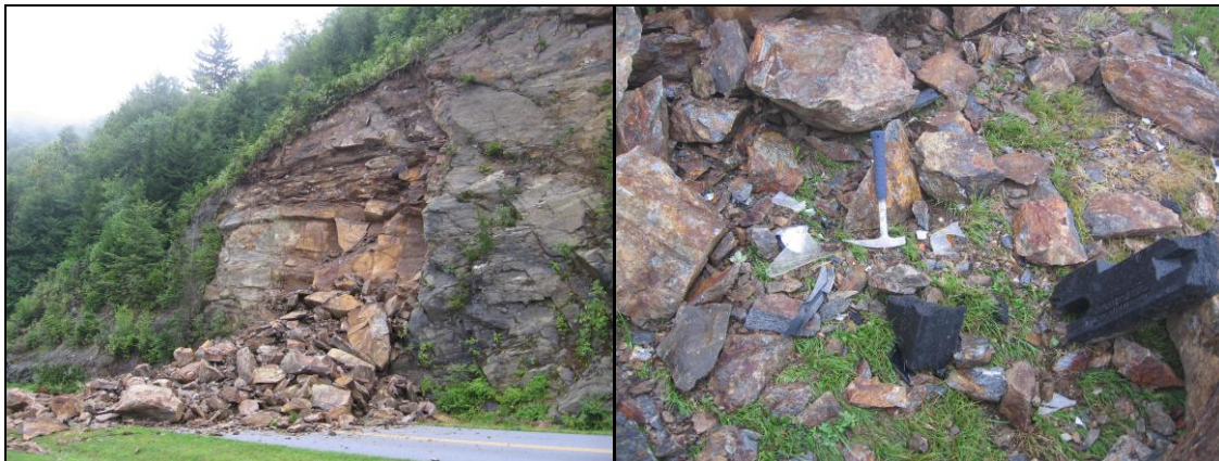
Figure B4. Left – August 18, 2006 rockslide (SNR-001) near the Cranberry Ridge overlook in metagraywacke and graphitic, sulfidic schist. NNP test values here range from -19.7 in schistose metagraywacke (SNR-001D), to -41.9 in graphitic sulfidic schist (SNR-001C) shown on Figure 1. Right – Close up view of broken rock fragments of rock slide debris with parts of the vehicle totaled in the slide. Iron oxide stained weathering surfaces and a dark gray sheen on the freshly exposed broken faces of the rock fragments typifies graphitic, sulfidic rocks.
