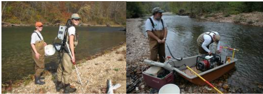
Figure 3. Backpack (left) and tow barge (right) electrofishing gear used in wadeable streams.
